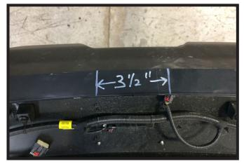
25. Using a reciprocating saw trim the rear fascia to allow clearance for the receiver hitch. Approximately 3-1/2" wide by 2" deep.
