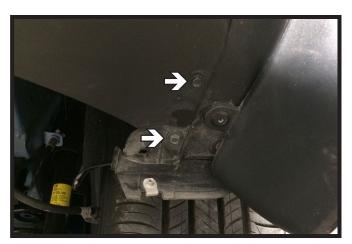
12. Using a 7MM socket, remove the two (2) bolts from behind the tire. Do this on both sides of the vehicle.
