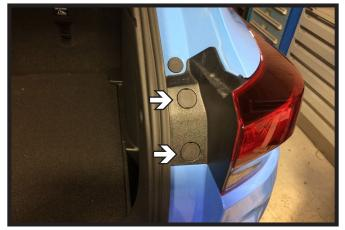
1. Remove the two (2) plastic caps next to the tail light. Do this on both sides of the vehicle.
