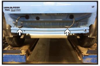
16. Unclip the wire loom from the bumper on each side of the vehicle.
