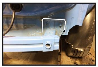
15. Using a utility knife or razor blade, cut around the bumper where it attaches to the frame.
