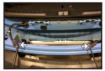
As the rear fascia is removed, unplug the two (2) electrical connections. There is one (1) on each side of the vehicle. Remove the fascia and set aside to be reinstalled later.
