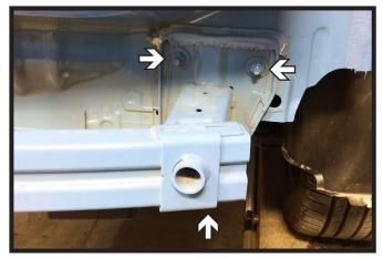
17. Using a 15MM socket, remove the three(3) nuts from the rear bumper. Do this on both sides of the vehicle. Remove bumper and set aside to be reinstalled later.
