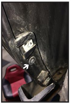
7. Using a 7MM socket, remove the one (1) bolt underneath the mud flap. Do this on both sides of the vehicle.
