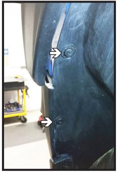
5. Using a T15 Torx, remove the two (2) bolts from the edge of the wheel well. Do this on both sides of the vehicle.
