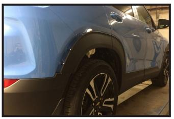
8. Pull back the rear wheel well trim past the fascia joint. Prop trim away from the vehicle using a soft cloth. Do this on both sides of the vehicle.
