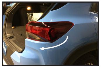
3. Push tailing toward the rear, remove and let hang. Do this on both sides of the vehicle.
