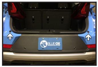
4. Using a T15 Torx, remove the two (2) bolts from the below the trail light housing. There is one (1) on each side of the vehicle.
