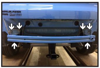
20. Place the rear bumper onto the vehicle. Reinstall the six (6) existing nuts and tighten.
