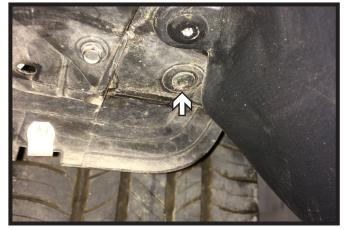
13. Using a T15 Torx, remove the one (1) bolt from behind the tire. Do this on both sides of the vehicle.
