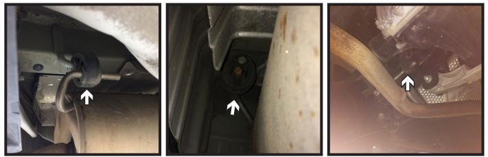
1. Support exhaust using a jack or stand. Remove the three (3) rubber isolators from exhaust rods. If the vehicle has a dual exhaust, remove the two (2) rubber isolators from the other side of the vehicle. Lower exhaust to allow receiver hitch installation.
