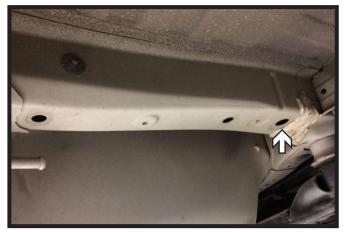
4. Using a die grinder, expand the access holes in the frame to 1-1/8". Do this on both sides of the vehicle.
