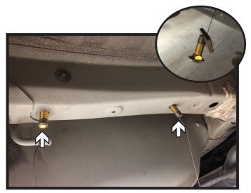
5. Feed lead wire from furthest existing frame hole to the access hole. Place spacer plates onto wire then attach lead wire to the end of the 1/2" carriage bolt (inset). Pull bolt and spacer plate through the frame. Repeat process with second bolt hole. Ensure spacer plates are sitting flush against inner frame and the bolts are hanging vertically. Do this on both sides of the vehicle.
