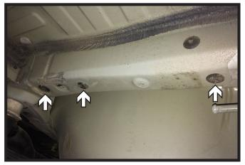
3. Remove the three (3) rubber plugs from the bottom of the frame. Do this on both sides of the vehicle.
