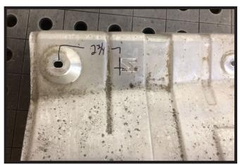
6. Measure 2-3/4" from the forward existing hole in the heat shield. Using a 1-1/2" hole saw, drill a hole in the heat shield in line with the existing holes. Repeat this step on second heat shield if present.
