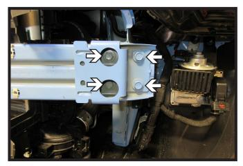
Using a 15MM socket, remove the four
