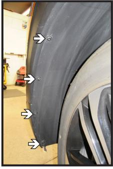
2. Using a T15 Torx, remove the four (4) bolts from the wheel well edge. Do this on both sides of the vehicle.
