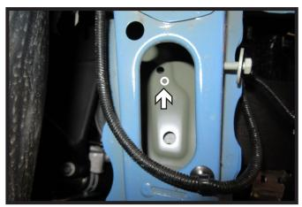
20. Hold the support plate in place as shown on passenger side of the vehicle so the front holes and back bottom hole line up with the existing holes on the vehicle.
