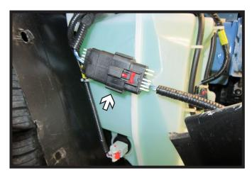
7. As the fascia is removed, disconnect the one (1) electrical connection on the passenger side of the vehicle. Set fascia aside to be reinstalled later.
