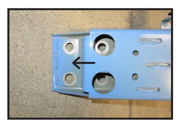
14. If needed, use a reamer to slot the four (4) holes 1/8" to 1/4" on the bumper towards the outside. Do this on both sides of the bumper.
