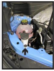
13. Using a 10MM socket, remove the two (2) nuts (white), one (1) bolt (gray), and one (1) push pin (black) from the windshield washer fluid reservoir on the passenger side of the vehicle. Disconnect the two (2) electrical connections. Then disconnect and plug all lines. Remove reservoir and set aside to be reinstalled later.
