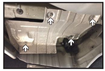
Using a 10MM socket, remove the four (4) bolts from the heat shield. Remove heat shield and set aside to be reinstalled later. Repeat this step on the other side of the vehicle if a second heat shield is present.
