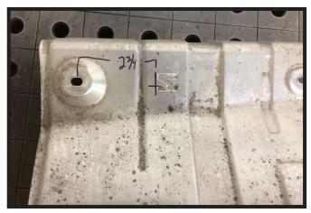
Measure 2-3/4" from the forward existing hole in the heat shield. Using a 1-1/2" hole saw, drill a hole in the heat shield in line with the existing holes. Repeat this step on second heat shield if present.
