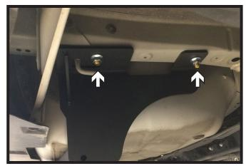
7. Raise hitch into position. Remove lead wires and loosely install 1/2" whiz flange nut onto each bolt. Then tighten all bolts.
