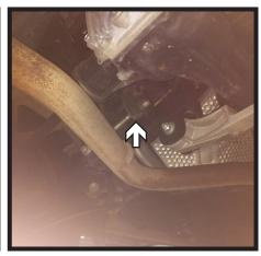
1. Support exhaust using a jack or stand. Remove the three (3) rubber isolators from exhaust rods. If the vehicle has a dual exhaust, remove the two (2) rubber isolators from the other side of the vehicle. Lower exhaust to allow receiver hitch installation.
