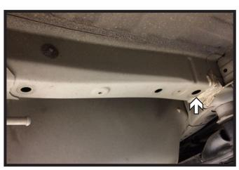
4. Using a die grinder, expand the access holes in the frame to 1-1/8". Do this on both sides of the vehicle.
