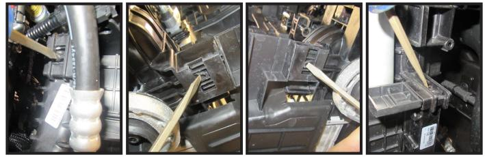
12. Using a flat screw driver, remove the four (4) clips attaching the bottom plastic shroud piece. Remove plastic piece, it will not be reinstalled.
