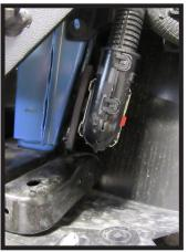
22. Reconnect electrical on passenger side and reattach electrical loom to frame on the driver side of the vehicle.
