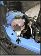
13. Using a 10MM socket, remove the two (2) nuts (white), one (1) bolt (gray), and one (1) push pin (black) from the windshield washer fluid reservoir on the passenger side of the vehicle. Disconnect the two (2) electrical connections. Then disconnect and plug all lines. Remove reservoir and set aside to be reinstalled later.
