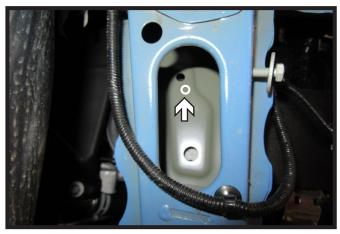
20. Hold the support plate in place as shown on passenger side of the vehicle so the front holes and back bottom hole line up with the existing holes on the vehicle. Mark frame using the baseplate as a template for top back hole. Using a 1/4" drill bit, create starter hole in frame. Then using a 1/2" drill bit, drill out top hole in frame.
