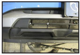
24. Using a reciprocating saw trim the horizontal slat on the fascia as shown to allow clearance for attachment tab and convenience link. Do this on both sides of the vehicle.
