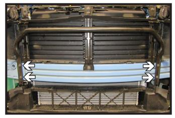
10. Using a 10MM socket, remove the four (4) bolts connecting the impact bar to the bumper. Set bar aside to be reinstalled later.
