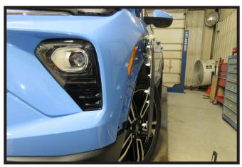
3. Pull back the wheel well trim, releasing the ten (10) push pins, past the fascia joint. Prop trim away from the vehicle using a soft cloth. Do this on both sides of the vehicle.
