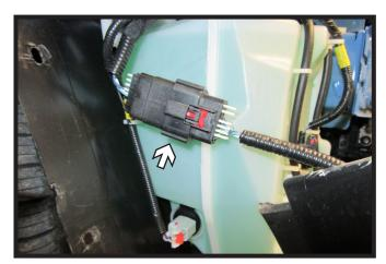
7. As the fascia is removed, disconnect the one (1) electrical connection on the passenger side of the vehicle. Set fascia aside to be reinstalled later.
