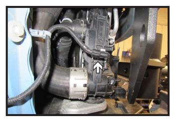
Unplug the electrical connection on the passenger side of the vehicle to allow for support plate installation. It will be reconnected later.
