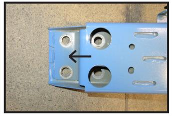
If needed, use a reamer to slot the four (4) holes 1/8" to 1/4" on the bumper towards the outside. Do this on both sides of the bumper.
