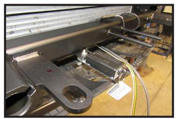
25. **Optional**: Using provided hardware, instal breakaway switch to the bracket on the baseplate as shown.
