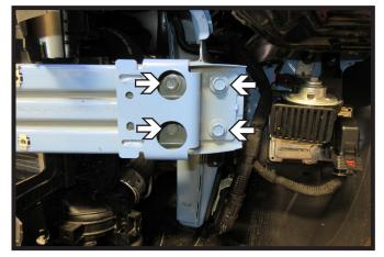
11. Using a 15MM socket, remove the four(4) bolts from the bumper. Do this on both sides of the vehicle. Remove bumper and set aside to be reinstalled later.
