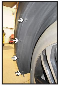
2. Using a T15 Torx, remove the four (4) bolts from the wheel well edge. Do this on both sides of the vehicle.
