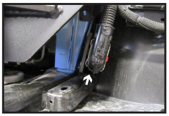
19. Unclip electrical loom from frame on driver side of the vehicle to allow for installation of support plate.
