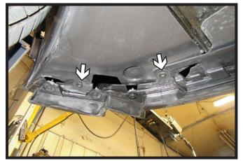
5. Using a T15 Torx, remove the two (2) bolts from the bottom of the fascia in front of the wheel. Do this on both sides of the vehicle.
