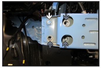
16. Slide the baseplate onto the vehicle between the frame and the bumper. Start one (1) existing 10MM bolt in the top outer hole (white). Do this on both sides of the vehicle. Level and center baseplate ensuring the holes on the bumper line up with the baseplate. Install the remaining three (3) existing bolts (gray) on each side of the vehicle.
