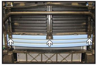
9. Using a 10MM socket, remove the three (3) bolts attaching the support brackets to the bumper
