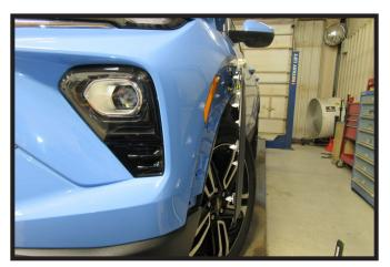
Pull back the wheel well trim, releasing the ten (10) push pins, past the fascia joint. Prop trim away from the vehicle using a soft cloth. Do this on both sides of the vehicle.
