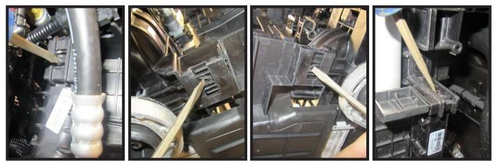
12. Using a flat screw driver, remove the four (4) clips attaching the bottom plastic shroud piece. Remove plastic piece, it will not be reinstalled.
