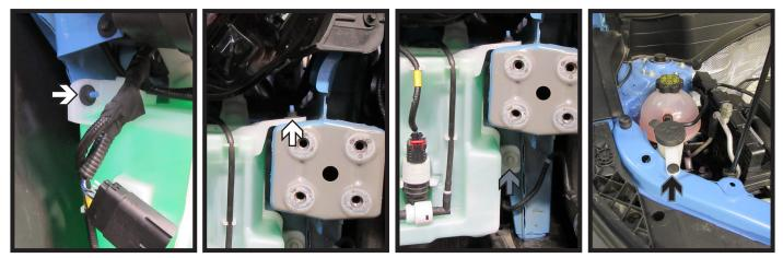
13. Using a 10MM socket, remove the two (2) nuts (white), one (1) bolt (gray), and one (1) push pin (black) from the windshield washer fluid reservoir on the passenger side of the vehicle. Disconnect the two (2) electrical connections. Then disconnect and plug all lines. Remove reservoir and set aside to be reinstalled later.
