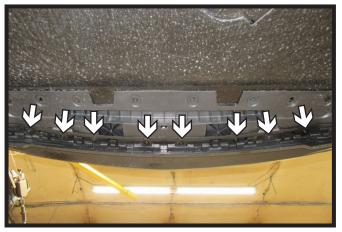
6. Using a 7MM socket, remove the eight (8) bolts from along the center on the under side of the fascia.
