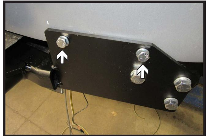
23. Install the two (2) 3/8" bolts with lock washers, flat washers, and nylon lock nuts. Do this on both sides of the vehicle.
