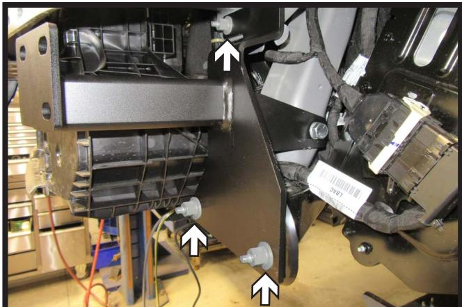
17. Slide the driver side baseplate piece onto the vehicle and start the three nuts. Leave loose at this time.
