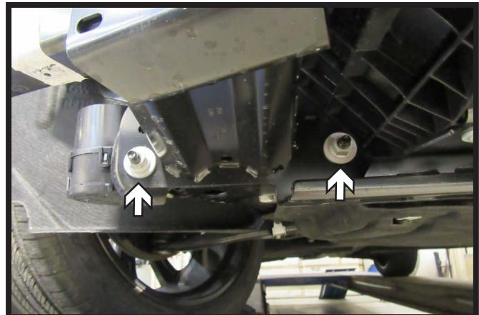
11. Using a 15MM socket, remove the two (2) nuts from behind the bottom bumper. Do this on both sides of the vehicle.
