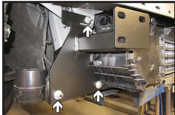
14. Slide the passenger side baseplate piece onto the vehicle and start the three (3) existing nuts. Leave loose at this time.
