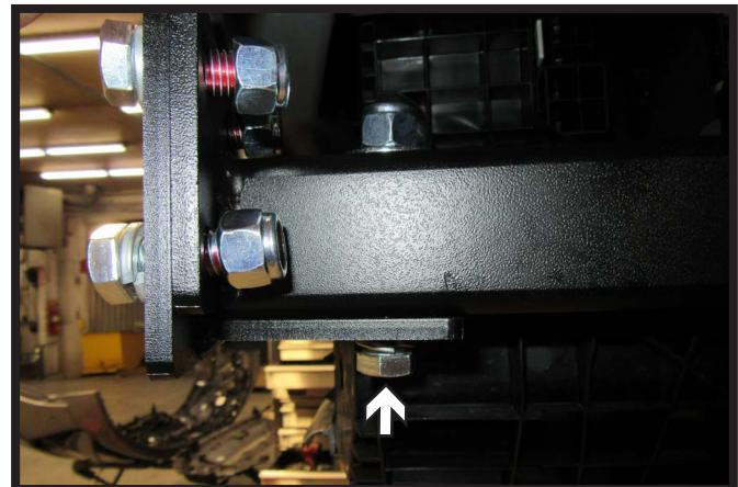
20. Start the one (1) 1/2" bolt in the bottom hole of the center piece with lock washer, flat washer, and nylon lock nut. Leave loose. Do this on both sides of the vehicle.
