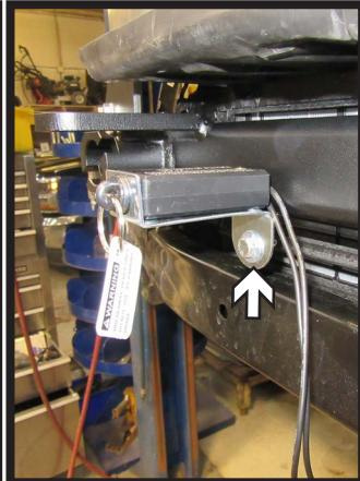
25. **Optional:** Using pliers and a vice grip bend the breakaway bracket as shown. Then using the provided 1/4" bolt with hex nut attach to the bracket on the passenger side of the baseplate.
