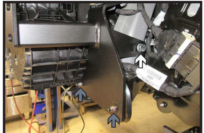
18. Using a 1/2" drill bit, drill hole in driver side of the frame using the baseplate as a template. Start the 1/2" bolt (white) with lock washer and whiz nut. Bend wire on whiz nut as needed and install through frame access hole. Leave loose at this time. Remove the nuts from the bottom two bolts (gray).
