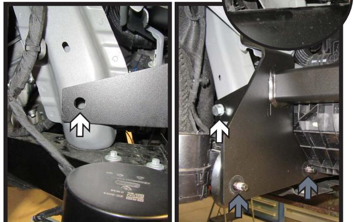
15. Using a 1/2" drill bit, drill out the hole on passenger of the frame using the baseplate as a template. Start the 1/2" bolt (white) with lock washer and whiz nut. Bend wire on whiz nut as needed and install through frame access hole (inset). Leave loose at this time. Remove the nuts from the bottom two bolts (gray).
