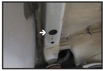
Measure 2" from the small hole on forward side of the vehicle and mark. Using a 1-1/8" hole saw, center and drill a access hole in the frame. Do this on both sides of the vehicle.
