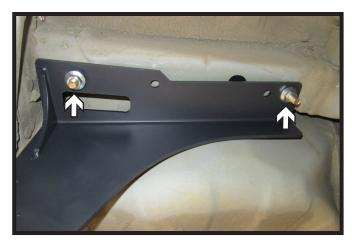
Raise hitch into position. Remove lead wires and loosely install 1/2" whiz flange nut onto each bolt. Then tighten all bolts.
