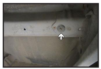
Remove the two (2) rubber plugs, one
