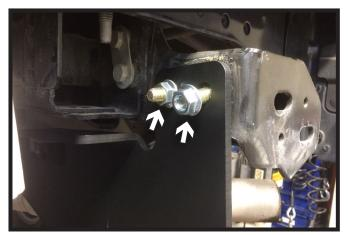
3. Raise the receiver hitch in place. Start the two (2) 1/2" bolts with flat washers and whiz nuts. Leave loose. Do this on both sides of the vehicle.
