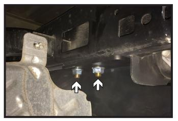
Start two (2) bolts with spacer plates and whiz lock nuts in the two forward holes. Leave loose. Do this on both sides of the vehicle.
