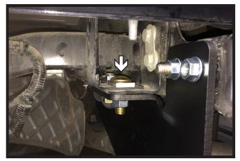
6. Start the one (1) bolt with spacer plate and whiz lock nut into the rear hole. Leave loose. Do this on both sides of the vehicle.
