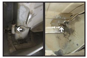
Remove the two (2) rear rubber isolators from the exhaust hangers to allow for easier heat shield removal. Set aside to be reinstalled later.
