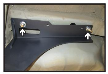
7. Raise hitch into position. Remove lead wires and loosely install 1/2" whiz flange nut onto each bolt. Do this on both sides of the vehicle. Then tighten all bolts.
