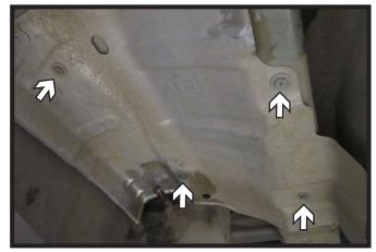
3. Using a 10MM socket, remove the four (4) bolts from the heat shield. Remove heat shield and set aside to be reinstalled later. Repeat this step on the other side of the vehicle if a second heat shield is present.
