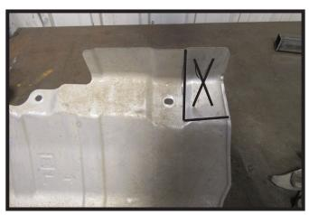
8. Hold heat shield(s) in place and mark as shown. Using a tin snip, trim the heat shield(s) to allow for receiver hitch clearance. Reinstall heat shield(s).
