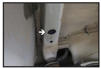
Measure 2" from the small hole on forward side of the vehicle and mark. Using a 1-1/8" hole saw, center and drill a access hole in the frame. Do this on both sides of the vehicle.
