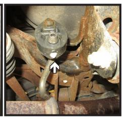
1. Support the exhaust and remove the three (3) rubber isolators from exhaust rods. Lower exhaust to allow receiver hitch installation.
