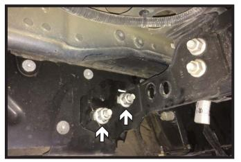
2. **Optional**: Using a 21MM socket, remove the two nuts from behind the bumper. Do this on both sides of the vehicle. Start to remove the rear bumper, unplug the two (2) electrical connections behind the bumper. Remove bumper and set aside to be reinstalled later.
