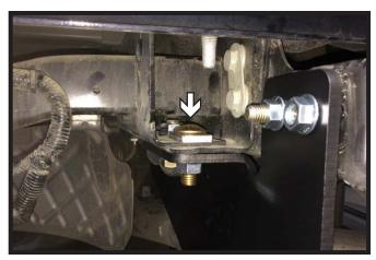
Start the one (1) bolt with spacer plate and whiz lock nut into the rear hole. Leave loose. Do this on both sides of the vehicle.
