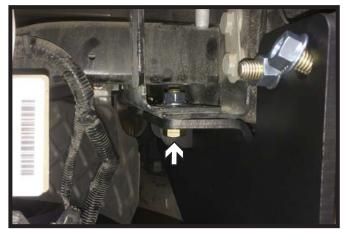
4. Start one (1) 5/8" bolt with flat washer and whiz nut into the second from the rear vertical hole. Leave loose. Do this on both sides of the vehicle.
