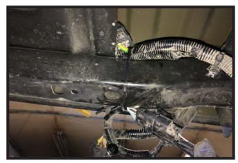
8. Using the provided zip ties, tie the wire looms to the frame.
