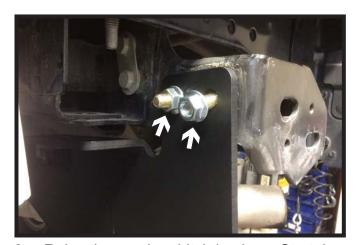
3. Raise the receiver hitch in place. Start the two (2) 1/2" bolts with flat washers and whiz nuts. Leave loose. Do this on both sides of the vehicle.
