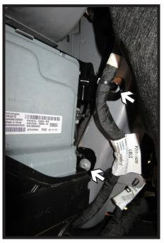
16. Using a 10MM socket, remove the one (1) nut from the top of the black box in front of the wheel on the driver side of the vehicle (left). Then remove the wire loom from the backside top bolt. Using a 10MM deep socket, remove the two (2) bolts from the backside (right). Let box hang out of the way for baseplate installation.
