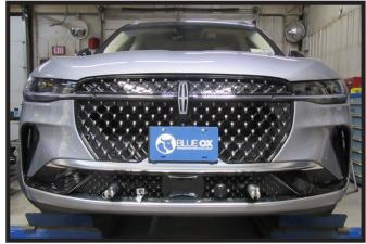
27. Reinstall the back box on the driver side of the vehicle. Then hold the fascia as close to its original position, mark and trim the fascia around the convenience links and attachment tabs. Reinstall the fascia and fascia cover and reconnect all electrical connections.
