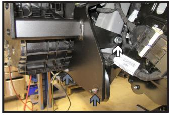
18. Using a 1/2" drill bit, drill hole in driver side of the frame using the baseplate as a template. Start the 1/2" bolt (white) with lock washer and whiz nut. Bend wire on whiz nut as needed and install through frame access hole. Leave loose at this time. Remove the nuts from the bottom two bolts (gray).
