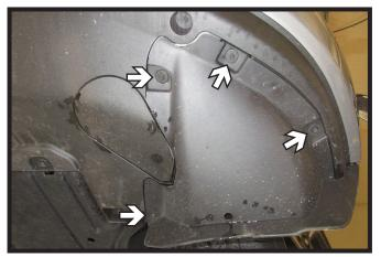
5. Using a 7MM socket, remove the four (4) bolts from the bottom of the fascia in front of the tire. Do this on both sides of the vehicle.
