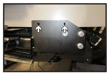
22. Using a 3/8" drill bit, drill out the two(2) holes in the top bumper using the baseplate as a template. Do this on both sides of the vehicle.
