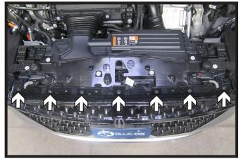
2. Using a 10MM socket, remove the seven (7) bolts from the top of the fascia.
