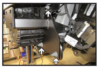
17. Slide the driver side baseplate piece onto the vehicle and start the three nuts. Leave loose at this time.
