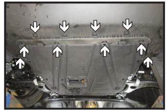
6. Using a 7MM socket, remove the ten (10) bolts from the bottom of the fascia in the center.
