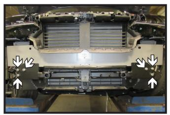
19. Hold baseplate center piece in place and start the three (3) 1/2" bolts with lock washers and nuts on each side of the vehicle, leave loose.
