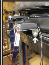
25. **Optional**: Using pliers and a vice grip bend the breakaway bracket as shown. Then using the provided 1/4" bolt with hex nut attach to the bracket on the passenger side of the baseplate.
