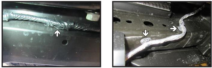
1. Unclip the wiring loom from the bumper and frame on the driver side of the vehicle. Let hang.
