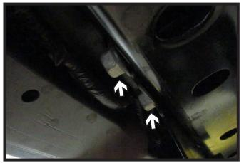
Using a 18MM socket, remove the two (2) bolts from the rear bracket behind the bumper. Remove bracket, it will not be reinstalled.
