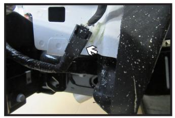
3. Unplug wire harness on passenger side of the vehicle.
