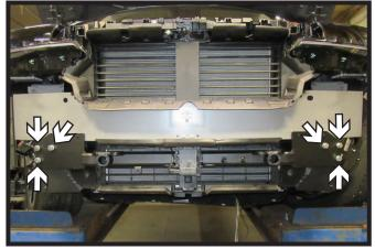
Hold baseplate center piece in place and start the three (3) 1/2" bolts with lock washers and nuts on each side of the vehicle, leave loose.
