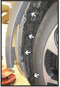
4. Remove the four (4) push pins from along the edge of the wheel well. Do this on both sides of the vehicle.
