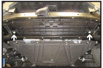
12. Using a 10MM socket, remove the two (2) bolts from the underside of the vehicle. Remove the bottom bumper and set aside to be reinstalled later.
