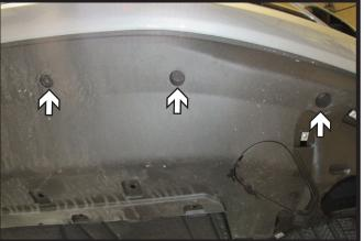
7. Using a 7MM socket, remove the six (6) bolts from along the front edge on the bottom of the fascia.
