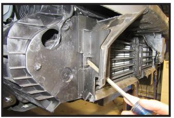
13. Using a reciprocating saw trim the shutter housing as shown. Then using a flat screw driver release the clip on each side of the shutter housing. Remove the trimmed pieces of the housing.
