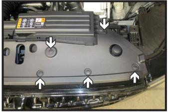
1. Remove the ten (10) push pins from the top of the fascia, there are five (5) on each side of the vehicle. Remove fascia cover and set aside to be reinstalled later.
