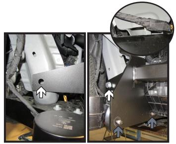
15. Using a 1/2" drill bit, drill out the hole on passenger of the frame using the baseplate as a template. Start the 1/2" bolt (white) with lock washer and whiz nut. Bend wire on whiz nut as needed and install through frame access hole (inset). Leave loose at this time. Remove the nuts from the bottom two bolts (gray).
