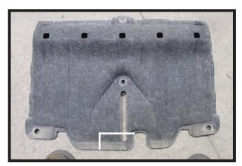
8. If needed, using snips, trim the underbody panel as shown to allow clearance for receiver hitch. Reinstall panel.
