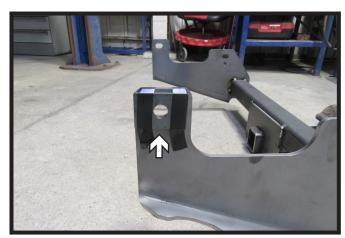
4. On the outside of the hitch, center the 1-3/4" x 2-1/2" x 1/4" spacer plate over the front hole of the receiver hitch. Tape in place to allow for easier installation. Do this on both sides of the receiver hitch.
