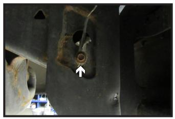
If present, using a 10MM socket, remove the one (1) bolt attaching the grounding cable to the passenger side frame rail.
