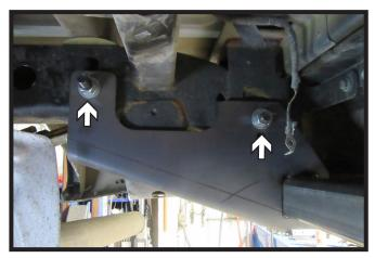
Slide receiver hitch into position and pull lead wired through the two (2) holes in the hitch. Do this on both sides of the vehicle.
