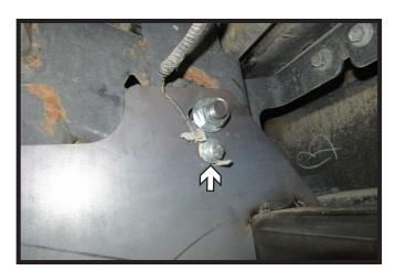
Reinstall grounding wire to the passenger side of the vehicle using the provided 8MM bolt with flat washer and lock washer. Tighten all bolts at this time.
