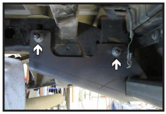
Slide receiver hitch into position and pull lead wired through the two (2) holes in the hitch. Do this on both sides of the vehicle.
