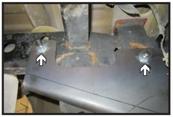
7. Carefully remove lead wire from bolts and loosely install flat washer and lock nut onto each of the four (4) bolts.
