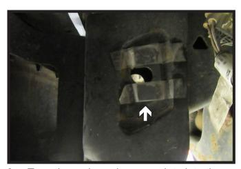
3. Tape the u-shaped spacer plate into the recess in the frame on the rear most hole. Do this on both sides of the vehicle.
