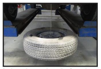
Lower the spare tire to allow for receiver hitch installation.
