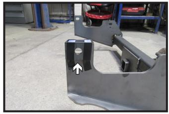
4. On the outside of the hitch, center the 1-3/4" x 2-1/2" x 1/4" spacer plate over the front hole of the receiver hitch. Tape in place to allow for easier installation. Do this on both sides of the receiver hitch.
