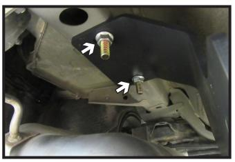
6. Raise receiver into place. Remove lead wire and carefully secure nuts to 1/2" bolts. Leave loose. Do this on both sides of the vehicle.
