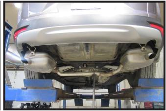
3. Remove three (3) rubber isolators from the exhaust rods at the rear of the vehicle. There is one (1) on each side and one (1) in the center. Support and lower exhaust.
