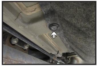
2. Remove the seven (7) push pins from the underbody panel. There are five (5) along the rear, one (1) in the center, and one (1) on the forward side. Remove panel and set aside to be reinstalled later.
