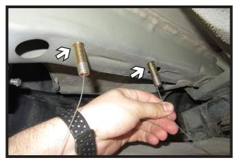
5. Pull bolts through the frame. Ensure the spacer plate is sitting flush against inner frame and the bolts are hanging vertically. Do this on both sides of the vehicle.
