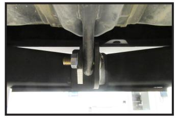
7. Insert the 1/2" x 2" bolt through the recovery loop and attach spacer plate and nut. Tighten all bolts at this time.
