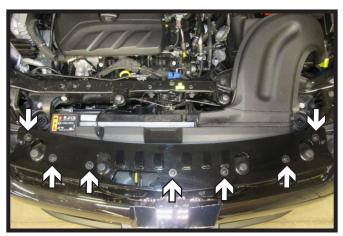
1. Using a T15 Torx, remove the seven (7) bolts from the top edge of the fascia.
