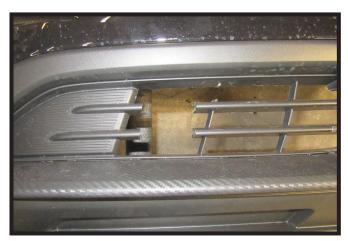
25. Using a reciprocating saw trim the fascia as shown to allow clearance for attachment tab and convenience link. Do this on both sides of the vehicle.
