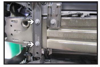
Using a 10MM socket, remove the two (2) bolts on each side connecting the impact bar to the bumper. Set bar aside to be reinstalled later.
