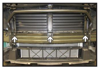
Using a 10MM socket, remove the three
