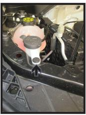
12. Using a 10MM socket, remove the two (2) nuts (white), one (1) bolt (gray), and one (1) push pin (black) from the windshield washer fluid reservoir on the passenger side of the vehicle. Disconnect the two (2) electrical connections. Then disconnect and plug all lines. Remove reservoir and set aside to be reinstalled later.
