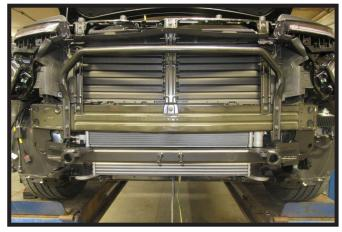
17. Reinstall the impact bar onto the bumper and tighten support bracket bolts. Then reinstall bolts attaching top shutters to bumper.
