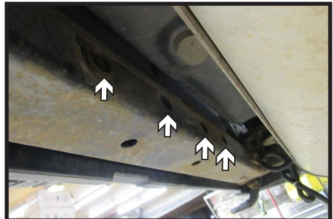
1. **Standard Models:** Support exhaust and remove rubber isolator from exhaust rod on each sides of the vehicle (above). Lower the exhaust to allow for easier receiver hitch installation.
