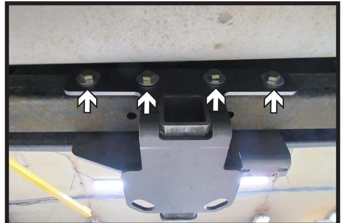
4. Install four (4) 1/2" bolts from the back side of the cross member with flat washers and whiz nuts.
