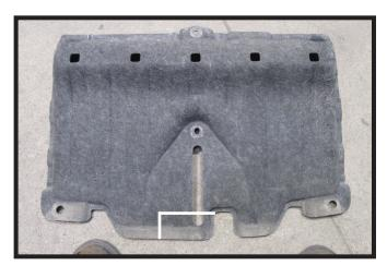
8. Using snips, trim the underbody panel as shown to allow clearance for receiver hitch. Reinstall panel.
