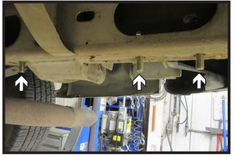
2. Slide spacer plates onto bolts and insert three (3) 1/2" bolts through existing frame holes as shown. Do this on both sides of the vehicle.
