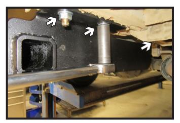
3. Raise receiver hitch into position and install the 1/2" flange nuts onto bolts. Do this on both sides of the vehicle.
