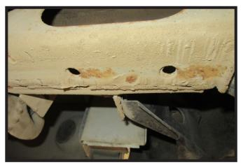
Clean away any debris or dirt from inside the frame and around existing holes so spacer plate will sit flush against frame when installed. Do this on both sides of the vehicle.
