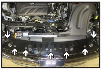
1. Using a T15 Torx, remove the seven (7) bolts from the top edge of the fascia.
