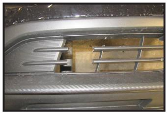
25. Using a reciprocating saw trim the fascia as shown to allow clearance for attachment tab and convenience link. Do this on both sides of the vehicle.
