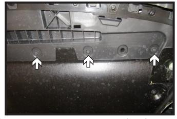
6. Using a 7MM socket, remove the six (6) bolts from the center on the under side of the fascia.
