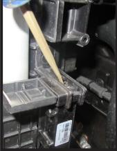
13. Using a flat screw driver, remove the four (4) clips attaching the bottom plastic shroud piece. Remove plastic piece, it will not be reinstalled.
