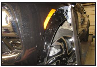
Pull back the wheel well trim, releasing the ten (10) push pins, past the fascia joint.
