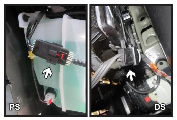
7. As the fascia is removed, disconnect the one (1) electrical connection on the passenger side and the one (1) on the driver side of the vehicle. Set fascia aside to be reinstalled later.
