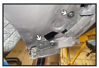
5. Using a T15 Torx, remove the two (2) bolts from the bottom of the fascia in front of the wheel. Do this on both sides of the vehicle.
