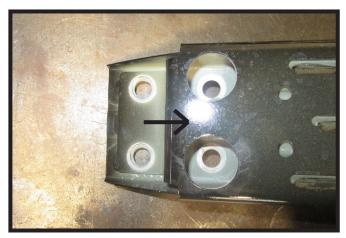
14. If needed, use a reamer to slot the four (4) holes 1/8" to 1/4" on the bumper towards the inside. Do this on both sides of the bumper.
