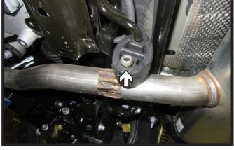
3. **Optional/Some Models**: Support center exhaust pipe using a jack or bungee cord. Then remove rubber isolator from exhaust rod.
