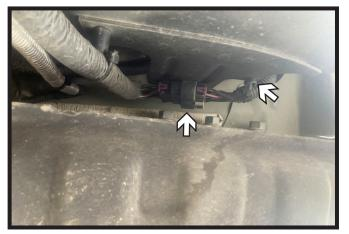
1. **Diesel Models**: Unclip the electrical connection on the passenger side of the vehicle. Then slid clips off of the rear studs securing the DEF tank.
