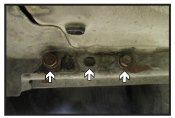
Using a 21MM socket, remove the two (2) or three (3) M14 bolts depending on vehicle model. Do this on both sides of the vehicle. Set bolts aside to be used for receiver hitch installation.
