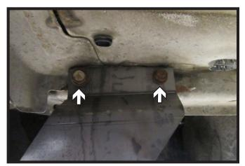
6. Raise receiver hitch into place and reinstall the two (2) M14 bolts. Do this on both sides of the vehicle.
