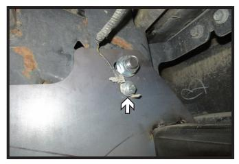
8. Reinstall grounding wire to the passenger side of the vehicle using the provided 8MM bolt with flat washer and lock washer. Tighten all bolts at this time.
