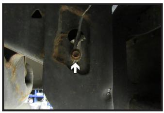
1. If present, using a 10MM socket, remove the one (1) bolt attaching the grounding cable to the passenger side frame rail.
