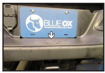
7. Reinstall trailer ball hole cap.
