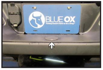
2. Remove the trailer ball hole cap for the center of the bumper.
