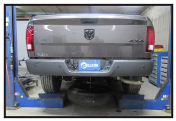
1. If needed, lower spare tire to allow for easier installation.
