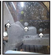
5. Using a T15 Torx, remove the nine (9) bolts from the bottom of the fascia. There are three (3) on each side in front of the tire and three (3) in the center. Do this on both sides of the vehicle.
