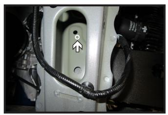
16. Using a 1/4" drill bit, create starter hole in frame on the passenger side of the vehicle. Then using a 1/2" drill bit, drill out top hole in frame.
