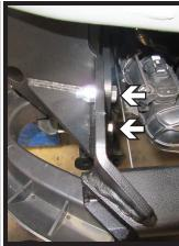
17. Slide support plate onto the vehicle toward the inside of the frame and baseplate. Start two (2) 3/8" bolts (white) with nylon lock nuts into front holes. Then start two (2) 1/2" bolts (gray) with lock washers, flat washers, and wire nuts in back holes. Tighten back 1/2" bolts then front 3/8" bolts. Do this on both sides of the vehicle.
