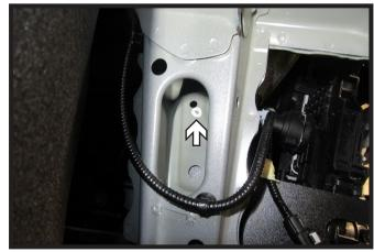
15. Hold the support plate in place on passenger side of the vehicle so the front holes and back bottom hole line up with the existing holes on the vehicle. Mark frame using the baseplate as a template for top back hole.
