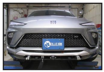
22. Hold the fascia as close to its original position, mark and trim the fascia around the convenience links and attachment tabs. Reinstall the fascia.
