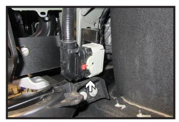
18. Reattach electrical loom to frame on the driver side of the vehicle.
