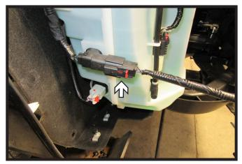
As the fascia is removed, disconnect the electrical connection on the passenger side of the vehicle. Set fascia aside to be reinstalled later
