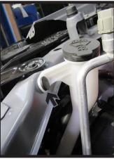
11. Using a 10MM socket, remove the two (2) nuts (white), one (1) bolt (gray), and one (1) push pin (black) from the windshield washer fluid reservoir on the passenger side of the vehicle. Disconnect the two (2) electrical connections. Then disconnect and plug all lines. Remove reservoir and set aside to be reinstalled later.
