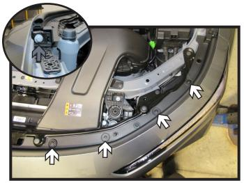
1. Using a T15 Torx, remove the four (4) bolts (white) from the top edge of the fascia. Then using a 10MM socket, remove the one bolt (gray, inset). Do this on both sides of the vehicle.
