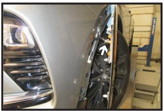
3. Pull back the wheel well trim, releasing the four (4) push pins, past the fascia joint. Disconnect the one (1) electrical connection. Prop trim way from the vehicle using a soft cloth. Do this on both sides of the vehicle.
