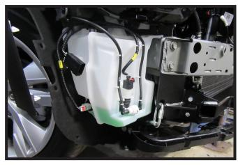
20. Reinstall windshield washer fluid reservoir, reconnecting all lines.
