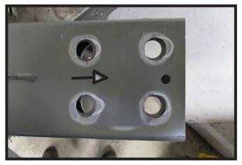
10. On the backside of the bumper slot the four (4) holes 1/8" to 1/4" as needed towards the outside. Do this on both sides of the bumper.
