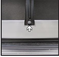
9. Using a 15MM socket, remove the four (4) bolts (right) from the bumper. Remove the one (1) push pin (center) from the back of the shroud above the bumper. Do this on both sides of the vehicle. Then using a 10MM socket, remove the one (1) bolt (left) from the support bracket in the center of the vehicle. Remove bumper and set aside to be reinstalled later.
