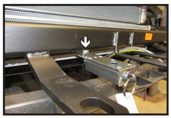
21. **Optional**: Mount the breakaway switch to the breakaway bracket with the provided 1/4" bolt and nut before reinstalling the fascia
