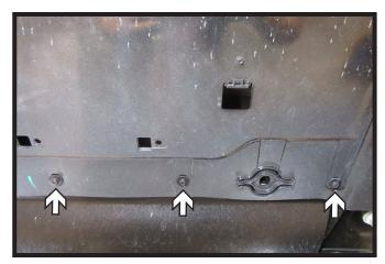
6. Using a 7MM socket, remove the six (6) bolts from the underside of the fascia.
