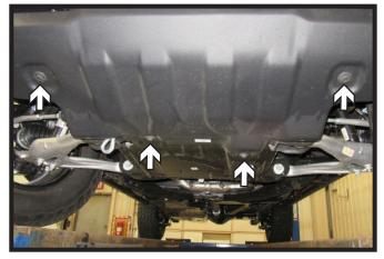
Using a 15MM socket, remove the four
