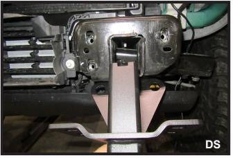
Slide the baseplate into the frame. Do this on both sides of the vehicle.
