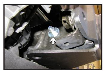
3b. **Baseplates Made After (4/12/23)**: Install the one (1) 1/2" bolt with flat washers, lock washer, and nut. Do this on both sides of the vehicle.
