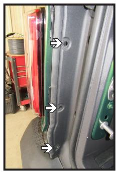
Using a Phillip's screw driver, remove the three (3) push pins. Unsnap black plastic piece. Do this on both sides of the vehicle.
