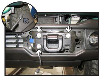
Using a 15MM socket, remove the three
