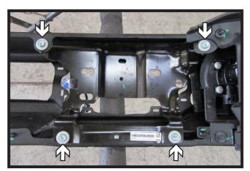
Using a 13MM socket, remove the four (4) bolts holding the D-ring bracket onto the bumper. Set bracket aside to be reinstalled on the bumper later. Do this on both sides of the vehicle.
