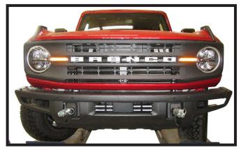
9a. Reinstall belly pan. Hold tow hook cover as close to its original position, mark and trim the covers as needed. Reinstall the covers.
