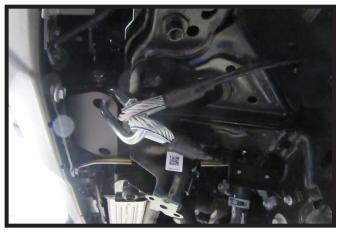
6. Attach the permanent baseplate safety cables to the provided convenience link on the baseplate. The photo above shows the recommended installation of the cables to frame of vehicle. Additional options may interfere with suggested mounting; in this case, secure the cables to a solid piece of the frame as described in the General Information sheet. Be sure the safety cables do not rub against any hoses or moving parts. Do this on **BOTH** sides of the vehicle. Reinstall belly pan.
