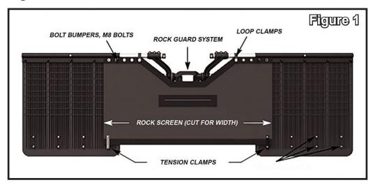
3. Remove pertinent Bolt Bumpers from the M8 Flap Clamp Bolts using a flat head screwdriver, if in use.
