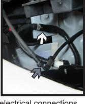
9. Unplug the two (2) electrical connections (white) on the passenger side of the vehicle. Then unplug the one (1) electrical connection (white) and one (1) hose line (gray) on the driver side of the vehicle.
