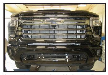
23. Reinstall bumper, grille, fascia, fascia cover and handle. Reconnect all electrical connections and hoses.
