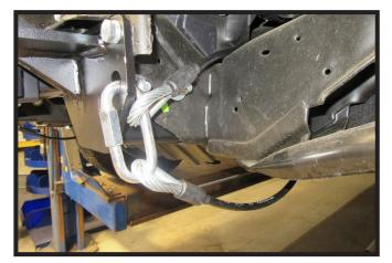
20. Attach the permanent baseplate safety cables to the provided convenience link on the baseplate. The photo above shows the recommended installation of the cables to frame of vehicle. Additional options may interfere with suggested mounting; in this case, secure the cables to a solid piece of the frame as described in the General Information sheet. Be sure the safety cables do not rub against any hoses or moving parts. Do this on **BOTH** sides of the vehicle.
