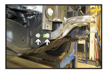
14. Using an 18MM socket and a wrench, remove the two (2) bolts from the tow hook. Do this on both sides of the vehicle. Remove tow hooks, they will not be reinstalled.
