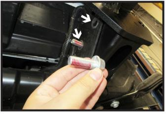
15. Slide baseplate onto vehicle so that the convenience link is to the outside of the vehicle (left). To ensure holes line up, start the four (4) 1/2" x 1-1/2" whiz flange bolts (right). Do this on both sides of the vehicle.
