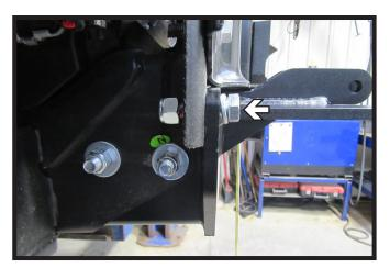
19. Install the two (2) 1/2" x 1-3/4" bolts with lock washers and nylon lock nuts into the front holes of the baseplate. Do this on both sides of the vehicle.
