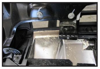
21. Using a reciprocating saw, trim the metal bracket on the back of the bumper as shown. Do this on both sides of the vehicle.
