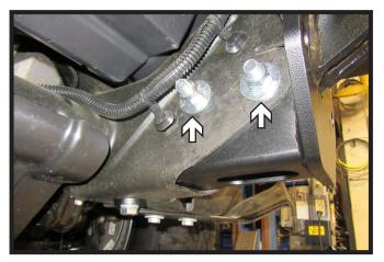
17. Install a flat washer and a nylon lock nut onto each of the four (4) 1/2" side bolts. Tighten the bottom bolt on the baseplate, the outside bolts, then inside bolts. Do this on both sides of the vehicle.
