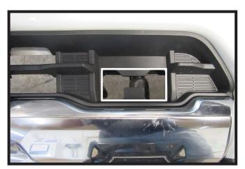
22. Using a reciprocating saw, trim the tow hook opening as shown to allow room for the baseplate. Do this on both sides of the vehicle.
