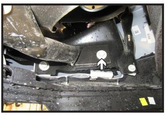
11. Using a 15MM socket, remove the one(1) bolt from the corner on the underside of the fascia. Do this on both sides of the vehicle
