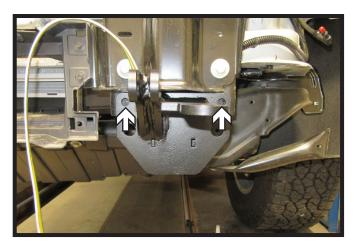
18. Using a 1/2" drill bit, drill out the front two (2) holes in the frame using the baseplate as a template. Do this on both sides of the vehicle
