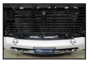
12. Using an 18MM socket, remove the two (2) bolts from the top edge of the bumper. Then remove plastic cover.
