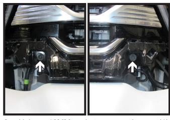
8. Using a 10MM socket, remove the one (1) bolt from the bottom corner of the grille on each side of the vehicle.
