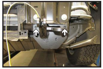
Using a 1/2" drill bit, drill out the front two (2) holes in the frame using the baseplate as a template. Do this on both sides of the vehicle.
