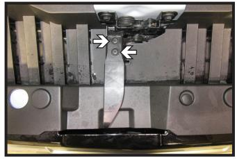
1. Using a T15 Torx, remove the two (2) bolts from the handle. Remove handle and set aside to be reinstalled later.
