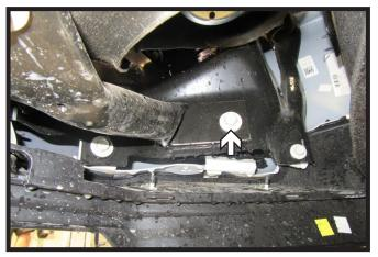
11. Using a 15MM socket, remove the one(1) bolt from the corner on the underside of the fascia. Do this on both sides of the vehicle.
