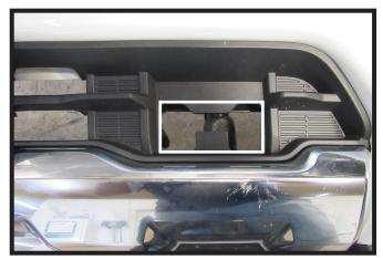
22. Using a reciprocating saw, trim the tow hook opening as shown to allow room for the baseplate. Do this on both sides of the vehicle.
