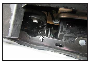
On the top side of the bumper, use an 18MM socket with socket extension to remove the one (1) bolt from behind the bumper. Do this on both sides of the vehicle. Remove bumper and set aside to be reinstalled later.
