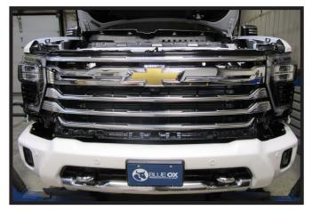
10. Grab the grille near the top and pull firmly away from the vehicle. Unsnap remaining clip near the bottom center of the grille. Remove grille and set aside to be reinstalled later.
