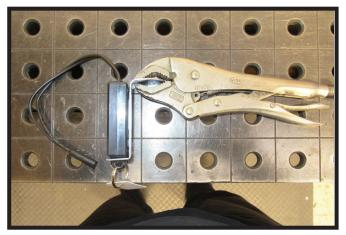
23. Optional Breakaway: Using a vise grip put a 90° bend in the breakaway switch, 1-1/2" from the back.
