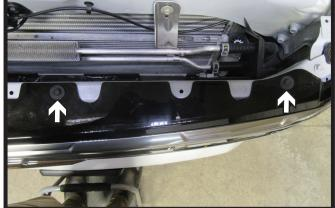
3. Using a 10MM socket, remove the four (4) bolts from the top of the fascia.
