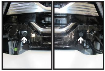
8. Using a 10MM socket, remove the one (1) bolt from the bottom corner of the grille on each side of the vehicle.
