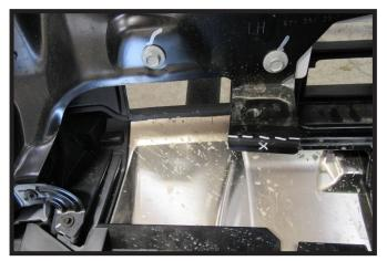
21. Using a reciprocating saw, trim the metal bracket on the back of the bumper as shown. Do this on both sides of the vehicle.
