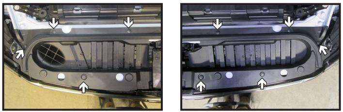
2. Remove the nine (9) push pins from the top of the fascia, there are five (5) on the driver side and four (4) on the passenger side of the vehicle. Remove fascia cover and set aside to be reinstalled later.
