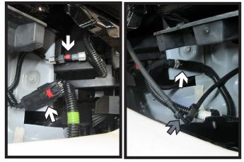
Unplug the two (2) electrical connections (white) on the passenger side of the vehicle. Then unplug the one (1) electrical connection (white) and one (1) hose line (gray) on the driver side of the vehicle.
