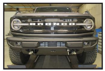
14. Reinstall the plastic pieces, bumper and skid plate. Reconnect all electrical connections.
