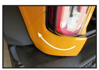
3. Carefully unsnap and remove plastic piece below tail light. Do this on both sides of the vehicle.
