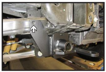
8. Using a 1/2" drill bit, drill the one (1) hole in the frame using the baseplate as a template. Do this on both sides of the vehicle.
