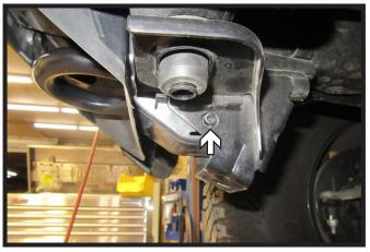
Pinch the back area of the plastic cover and remove from the tow hook, it will not be reinstalled. Do this on both sides of the vehicle
