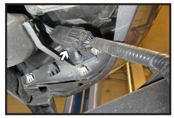
3. On the driver side of the vehicle, unplug the one (1) electrical connection from the underside of the vehicle. Remove bumper and set aside to be reinstalled later.
