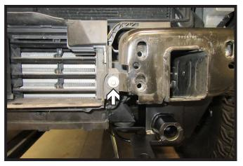
11. **Optional Breakaway**: Using a 8MM socket, remove the bolt from the driver side of the vehicle.
