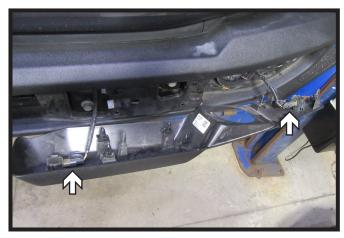
1. Pop plastic piece off of the bumper and disconnect the two (2) electrical connections. Set piece aside to be reinstalled later. Do this on both sides of the vehicle.
