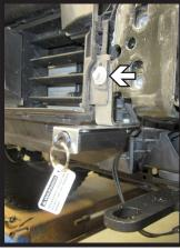
12. **Optional Breakaway**: Slide the breakaway bracket behind plastic piece and reinstall the existing bolt.
