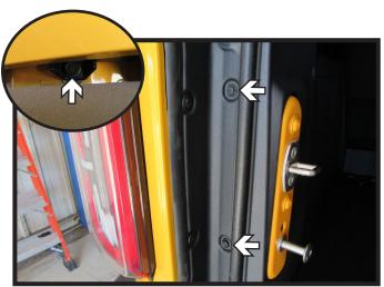
Using a 10MM socket, remove the three
