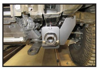
7. Slide the baseplate onto the vehicle. Start the two (2) existing bolts in the bottom holes of the baseplate. As the bolts are tightened, press inward and upward to lessen gap between baseplate ear and the frame. Do this on both sides of the vehicle.
