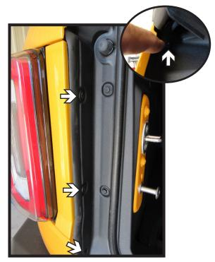
2. Using a Phillip's screw driver, remove the four (4) push pins. There are three (3) along the edge and one (1) at the top (inset). Unsnap black plastic piece and set aside to be reinstalled later. Do this on both sides of the vehicle.
