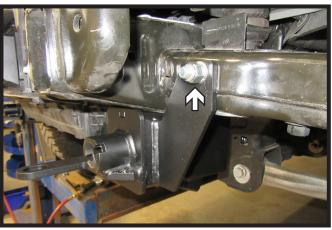
9. Using a 3/4" socket and wrench, install the one (1) 1/2" bolt with lock washer and nylon lock nut. Do this on both sides of the vehicle
