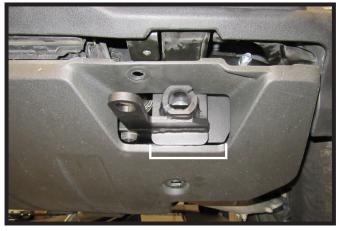
13. Hold the skid plate as close to its original position, mark and trim the skip plate around the convenience links and attachment tabs.
