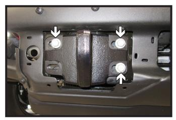
Using a 15MM socket, remove the three (3) bolts from the tow hook. Do this on both sides of the vehicle. Remove tow hooks with bumper and set aside to be reinstalled later. Tow hooks will not be reinstalled.
