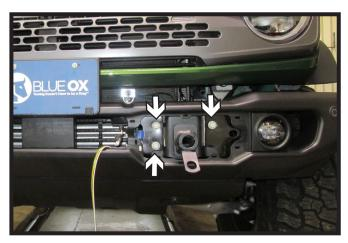
7. Slide bumper onto vehicle and reattach electrical on driver side. Then install the three (3) existing bolts. Do this on both sides of the vehicle.
