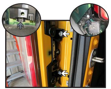
4. Using an 8MM socket, remove the two (2) bolts (white) and using a 10MM socket remove the two (2) bolts (gray, insets) attaching the tail light housing to the frame. Remove the tail light housing and install tail light wiring kit per kit instructions. Do this on both sides of the vehicle.
