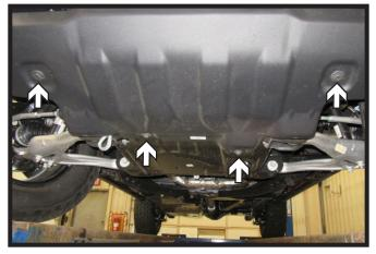
Using a 15MM socket, remove the four
