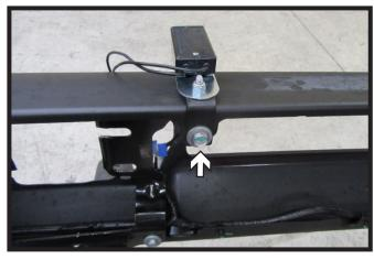
4. **Optional:** Attach the breakaway switch to the breakaway bracket using the provided one (1) 1/4" x 1" bolt with flat washer and nut (left). Then attach breakaway bracket with switch to the bumper on the driver side of the vehicle using the existing bolt and hardware (right).
