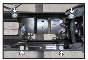
Using a 13MM socket, remove the four
