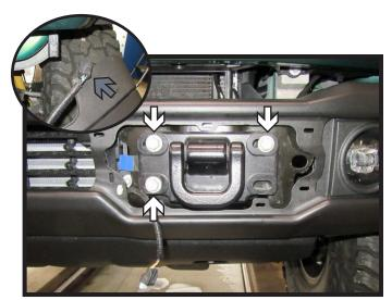
Using a 15MM socket, remove the three
