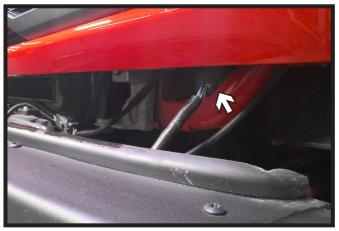
3. **Raptor Models**: As the bumper is removed, unplug the one (1) electrical connection on the driver side of the vehicle
