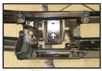
5. Using a 10MM socket, remove the one (1) bolt (white) from the tow hook bracket. Remove tow hook, it will not be reinstalled. Then using a 13MM socket, remove the four (4) bolts (gray) holding the tow hook bracket onto the bumper. Set bracket aside to be reinstalled on the bumper later. Do this on both sides of the vehicle.
