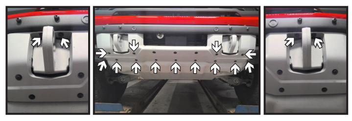
1b. **Raptor Models**: Remove the seventeen (17) push pins from plastic bumper cover. Pull on area around tow hooks to unsnap cover and remove. Set cover aside to be reinstalled later.
