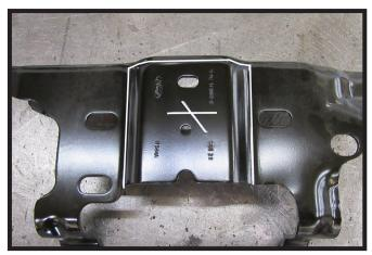
Using a reciprocating saw, cut and remove the indicated area of the tow hook bracket.
