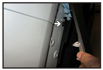
6. Using a 7MM socket, remove the one (1) bolt from the fascia joint. Do this on both sides of the vehicle.
