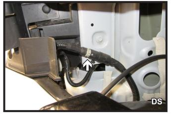
12. Unplug the one (1) electrical connection on the passenger side and one (1) on the driver side. Remove bumper and set aside to be reinstalled later.
