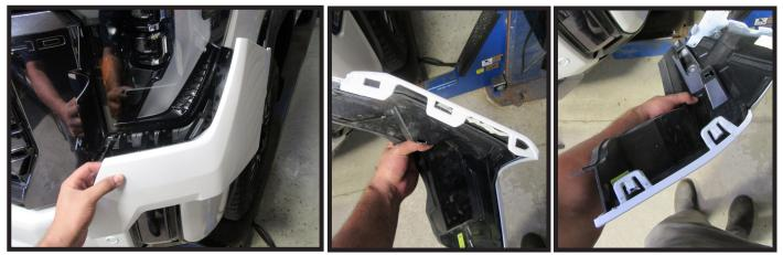
Remove the corner piece of the fascia by releasing the three (3) clips on the outside and two (2) clips toward the inside. Do this on both sides of the vehicle.
