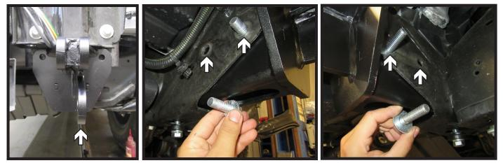
13. Slide baseplate onto vehicle so that the convenience link is to the outside of the vehicle (left). To ensure holes line up, start the two (2) 1/2" x 1-1/2" whiz flange bolts towards the inside (center) and the two (2) 1/2" x 2" with flat washer towards the outside of the vehicle (right). Do this on both sides of the vehicle.
