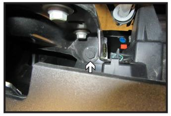
On the top side of the bumper, use an 18MM socket and socket extension to remove the two
