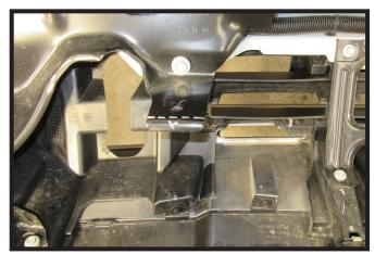
20. Using a reciprocating saw, trim the metal bracket on the back of the bumper as shown. Do this on both sides of the vehicle.
