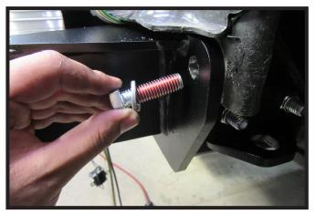
18. Install the two (2) 1/2" x 1-3/4" bolts with flat washers, lock washers, and nylon lock nuts into the front holes of the baseplate. Do this on both sides of the vehicle.
