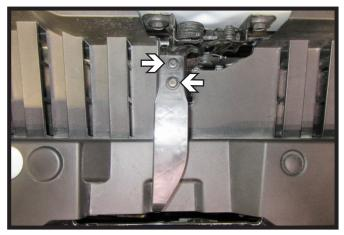
Using a T15 Torx, remove the two (2) bolts from the handle. Remove handle and set aside to be reinstalled later.
