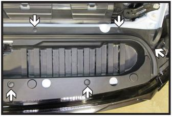
2. Remove the nine (9) push pins from the top of the fascia, there are five (5) on the driver side and four (4) on the passenger side of the vehicle. Remove fascia cover and set aside to be reinstalled later.
