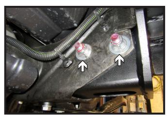
16. Install a flat washer and a nylon lock nut onto each of the two (2) 1/2" inside bolts. Fully tighten. Then tighten the bottom bolt on the baseplate. Do this on both sides of the vehicle.
