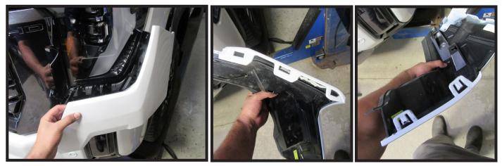
7. Remove the corner piece of the fascia by releasing the three (3) clips on the outside and two (2) clips toward the inside. Do this on both sides of the vehicle.
