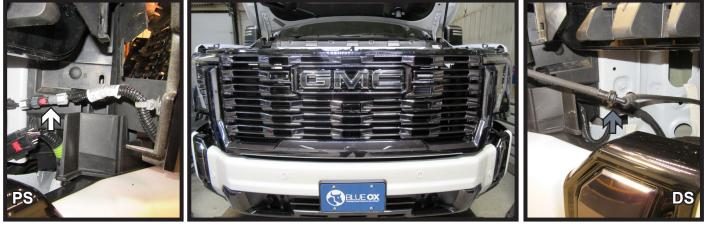
8. Start removing the grille piece by releasing the five (5) clips along the bottom, thee (3) on each side, and one (1) in the center under the emblem. Disconnect the one (1) electrical connection (white) on the passenger side and one (1) hose (gray) on the driver side. Remove and set grille aside to be reinstalled later.
