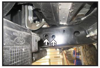
Before installing the baseplate, ensure the 5/8" x 6-1/2" bolts will go completely through the frame. Holes may not fully line up on each side of the frame. If not ream out holes as needed.
