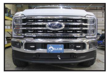
6. Hold bumper valance as close to it's original spot as possible and center on the vehicle. Mark and trim necessary clearance for baseplate, convenience links, and optional breakaway switch. Reinstall bumper valance.
