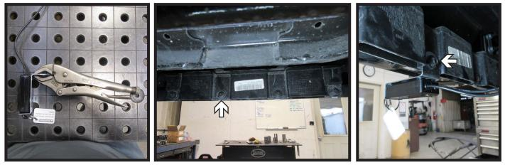
4. **Optional Breakaway**: Using a large vice grip, create a 90° bend as shown in the breakaway switch (left). Then using an 8MM socket remove one (1) of the four (4) bolts on the back side of the bumper (center). Install breakaway bracket to the back of the bumper using existing bolt (right).
