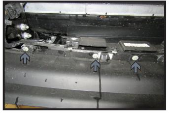
Using an 8MM socket, remove the thirteen (13) bolts from the lower bumper valance. There are three (3) bolts (white) on each end that are accessible from above and the other seven (7) bolts (gray) are accessible from below. Remove valance and set aside to be reinstalled later.
