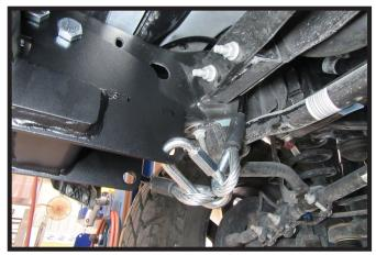
5. Attach the permanent baseplate safety cables to the provided convenience link on the baseplate. The photo above shows the recommended installation of the cables to frame of vehicle. Additional options may interfere with suggested mounting; in this case, secure the cables to a solid piece of the frame as described in the General Information sheet. Be sure the safety cables do not rub against any hoses or moving parts. Do this on **BOTH** sides of the vehicle.
