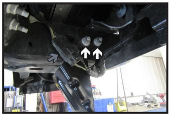
2. Using an 18MM socket, remove the four (4) nuts (white) and factory bolt hardware from the bracket. Remove bracket, it will not be reinstalled. Do this on both sides of the vehicle. Then remove push pin attaching the wire loom (gray) to the frame on the driver side of the vehicle.
