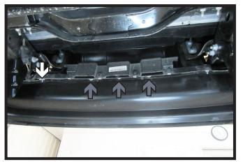
1. Using an 8MM socket, remove the thirteen (13) bolts for the lower bumper valance. There are five (5) bolts (white) on each side that are accessible from above and three (3) bolts (gray) along the center that are accessible from below. Remove valance and set aside to be reinstalled later.
