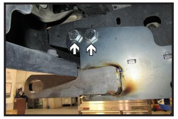
Slide baseplate onto vehicle with convenience link towards the center of the vehicle. Start the two (2) 5/8" x 6-1/2" bolts with nylon lock nuts. Do this on both sides of the vehicle. Do not fully tighten at this time.
