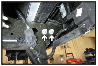
2. Using an 18MM socket, remove the four (4) nuts (white) and factory bolt hardware from the bracket. Do this on both sides of the vehicle. Remove brackets and set aside. They will not be reinstalled. Then remove push pin attaching the wire loom (gray) to the frame on the driver side of the vehicle.
