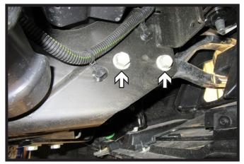
Using an 18MM socket and a wrench, remove the two (2) bolts from the tow hook. Do this on both sides of the vehicle. Remove tow hooks, they will not be reinstalled.
