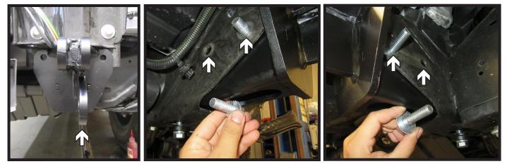
13. Slide baseplate onto vehicle so that the convenience link is to the outside of the vehicle (left). To ensure holes line up, start the two (2) 1/2" x 1-1/2" whiz flange bolts towards the inside (center) and the two (2) 1/2" x 2" with flat washer towards the outside of the vehicle (right). Do this on both sides of the vehicle.
