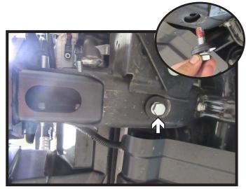
14. Start the bottom 1/2" x 1-3/4" bolt with lock washer, thick washer, and slotted plate. Press baseplate up and in while hand tightening the bolt. Do this on both sides of the vehicle.
