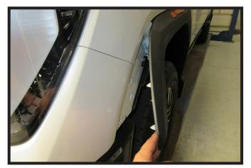
5. Pull back the wheel well trim past the fascia joint. Prop trim away from the vehicle using a soft cloth. Do this on both sides of the vehicle.
