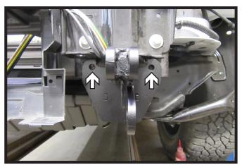
17. Using a 1/2" drill bit, drill out the front two(2) holes on the baseplate. Do this on both sides of the vehicle.
