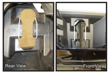
21. Using a reciprocating saw, trim the tow hook opening as shown to allow room for the baseplate. Do this on both sides of the vehicle.
