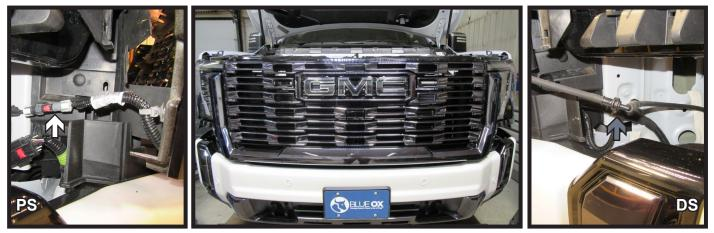
8. Start removing the grille piece by releasing the five (5) clips along the bottom, thee (3) on each side, and one (1) in the center under the emblem. Disconnect the one (1) electrical connection (white) on the passenger side and one (1) hose (gray) on the driver side. Remove and set grille aside to be reinstalled later.
