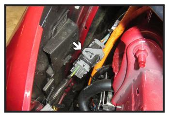
7. Disconnect the one (1) electrical connection on the passenger side of the vehicle.
