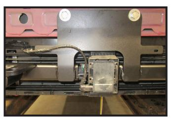
31. Reinstall the four (4) bolts attaching the ACC to the frame.
