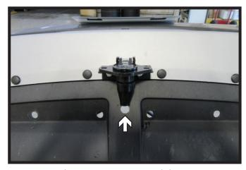
33. Center electrical bracket on bottom of the fascia. Using a 1/4" drill bit, drill two (2) holes using the bracket as a template. Install provided two (2) 1/4" bolts with hardware (left). Hold electrical plug in place and mark fascia below end of plug. Using a 5/8" drill bit, drill one (1) hole to feed tail light electrical wires through (right).
