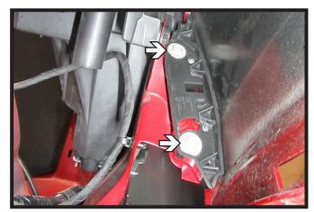
4. Pull back the wheel well liner. Using a 10MM socket, remove the two (2) bolts from the fascia joint. Do this on both sides of the vehicle.
