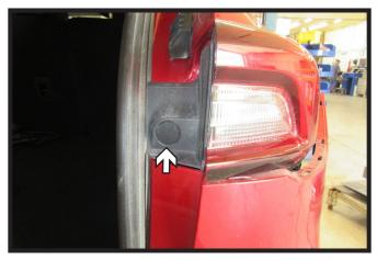
Remove the bolt cover from the tail light housing. Do this on both sides of the vehicle.
