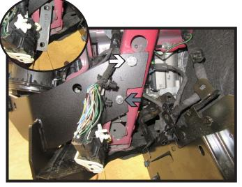
28. Insert nut plate through hole in the frame (inset). Insert a 1/2" bolt with lock washer into the top hole (white) and a 3/8" bolt with lock washer into the bottom hole (gray).
