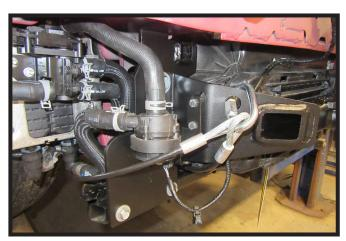
34. Attach the permanent baseplate safety cables to the provided convenience link on the baseplate. The photo above shows the recommended installation of the cables to frame of vehicle. Additional options may interfere with suggested mounting; in this case, secure the cables to a solid piece of the frame as described in the General Information sheet. Be sure the safety cables do not rub against any hoses or moving parts. Do this on BOTH sides of the vehicle
