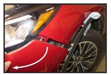
Remove fascia, set aside to be reinstalled later.
