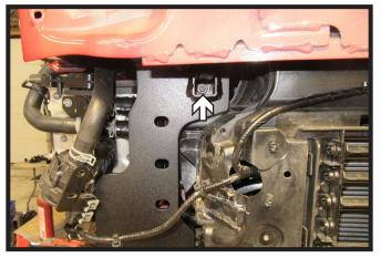
18. Reinstall the one (1) existing nut in to tube hole.
