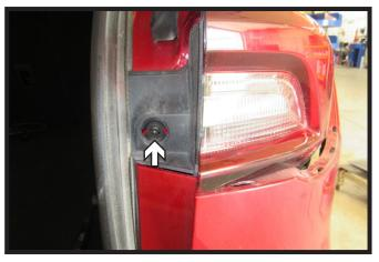
5. Using a T25 Torx, remove the two (2) bolts from the tail light housing. Remove housing and install tail light wiring kit per manufactures instructions. Reinstall tail light housing, rear panel and push pins. Do this on both sides of the vehicle.
