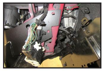
25. Remove the four (4) push pins attaching the electrical bracket and loom to the black box on the driver side of the vehicle.
