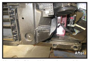
16. Using a reciprocating saw, shave the rib on the driver side of the vehicles as shown so it is flush with the shutter housing to allow clearance for the baseplate.
