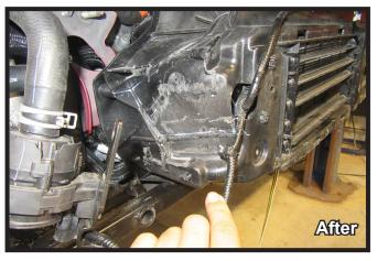
15. Using a reciprocating saw, shave the ribs on the passenger side of the vehicle as shown so they are flush with the shutter housing to allow clearance for the baseplate.
