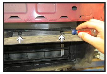
12. Remove the shroud around the lower shutters by removing the two (2) push pins, one (1) on each side of the vehicle. Then using a flat screw driver, remove the eight (8) clips around the edge of the shroud.
