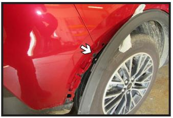
Pull back the wheel well trim and hold in place with a soft cloth. Remove the one
