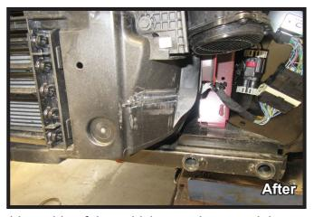
16. Using a reciprocating saw, shave the rib on the driver side of the vehicles as shown so it is flush with the shutter housing to allow clearance for the baseplate.
