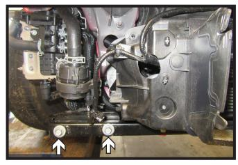
14. Using a 13MM socket, remove the two (2) bolts from the cross bar. Do this on both sides of the vehicle.
