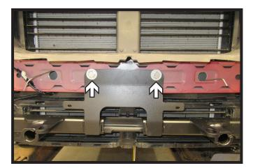
30. Install two (2) 1/2" bolts with washers and wire nuts. Torque bolts to 50 ft/lbs.
