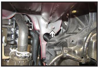
10. Using a 15MM socket with extension, remove the one (1) nut on the passenger side of the vehicle.
