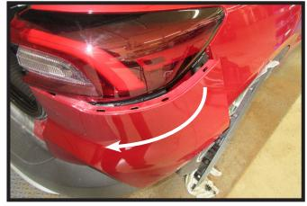
Remove the rear panel below the tail light housing. Do this on both sides of the vehicle.
