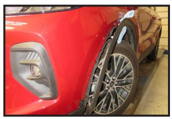
Pull back the wheel well trim past the fascia joint and hold in place with a soft cloth. Do this on both sides of the vehicle.
