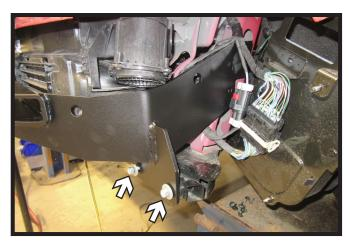
23. Ensure driver side plate is as close to the frame as possible then tighten bottom two (2) existing bolts. Then tighten the three (3) 1/2" bolts on the passenger side of the vehicle.
