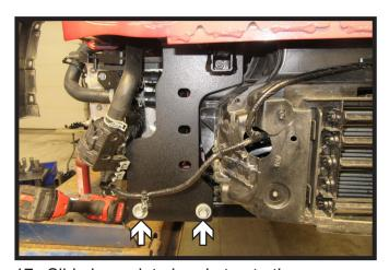
17. Slide baseplate bracket onto the passenger side of the vehicle and start two (2) of the existing 8MM bolts with washers into the bottom holes.
