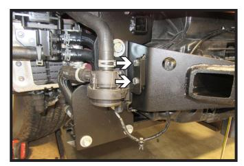
24. Using two (2) 1/4" x 1-1/4" bolts with nuts to attach bracket to the baseplate on the passenger side of the baseplate.
