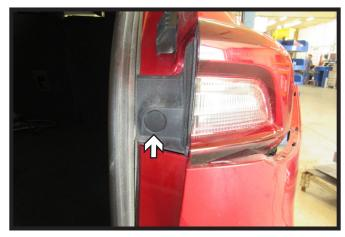
Remove the bolt cover from the tail light housing. Do this on both sides of the vehicle.
