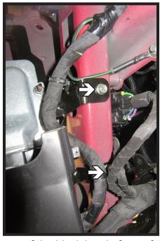
11. Using a 10MM socket, remove the one (1) bolt from the top of the black box in front of the wheel on the driver side of the vehicle (left). Then remove the wire loom from the backside bottom bolt. Using a 10MM deep socket, remove the two (2) bolts from the backside (right). Let box hang out of the way for baseplate installation.
