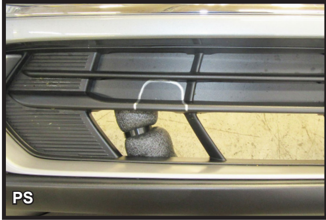
25a. Fascia Style 1: Using a reciprocating saw trim each side of the fascia as shown to allow room for the baseplate and convenience link.
