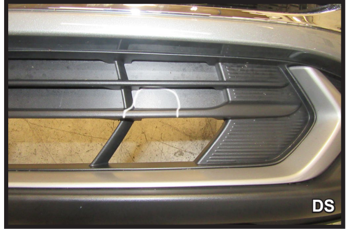
25a. Fascia Style 1: Using a reciprocating saw trim each side of the fascia as shown to allow room for the baseplate and convenience link.
