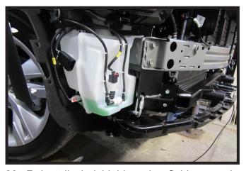
23. Reinstall windshield washer fluid reservoir, reconnecting all lines.
