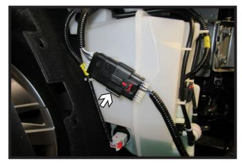
8. Disconnect the electrical connection on the passenger side of the vehicle.
