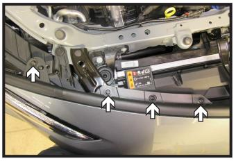
Using a T15 Torx, remove the four (4) bolts from the top edge of the fascia. Do this on both sides of the vehicle.
