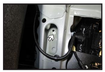
18. Using a 1/4" drill bit, create starter hole in frame on the passenger side of the vehicle. Then using a 1/2" drill bit, drill out top hole in frame.
