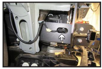
21. Reconnect electrical on the passenger side of the vehicle.
