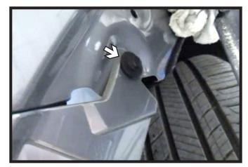
Using a 7MM socket, remove the one (1) bolt from the fascia joint. Do this on both sides of the vehicle.
