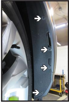
2. Using a T15 Torx, remove the four (4) bolts from along the edge of the wheel well. Do this on both sides of the vehicle.
