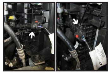
10. Unclip the electrical loom from the shroud on the passenger side of the vehicle (left). Then using a provided zip tie, connect the loom to the plastic behind the shroud as shown (right) so that it out of the way when removing the shroud piece.
