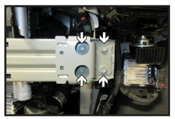
Using a 15MM socket, remove the four (4) bolts from the bumper. Do this on both sides of the vehicle. Let bumper hang from the support bracket.
