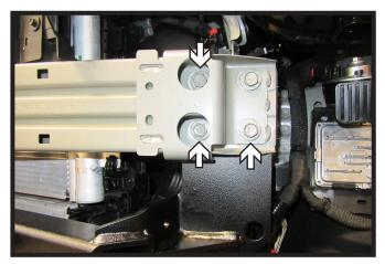
14. Start the remaining three (3) existing bolts. Do this on both sides of the vehicle. Ensure the baseplate is level and tighten all eight (8) bolts, four (4) on each side.
