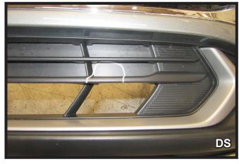
25a. **Fascia Style 1**: Using a reciprocating saw trim each side of the fascia as shown to allow room for the baseplate and convenience link.
