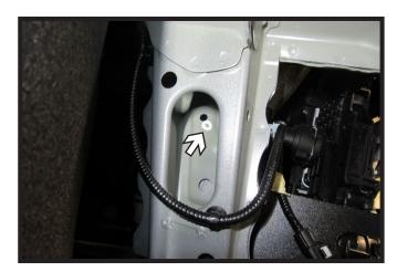
17. Hold the support plate in place on passenger side of the vehicle so the front holes and back bottom hole line up with the existing holes on the vehicle. Mark frame using the baseplate as a template for top back hole.
