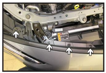
1. Using a T15 Torx, remove the four (4) bolts from the top edge of the fascia. Do this on both sides of the vehicle.
