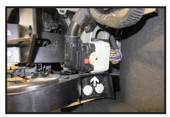
Unclip electrical loom from frame on driver side of the vehicle to allow for installation of support plate.
