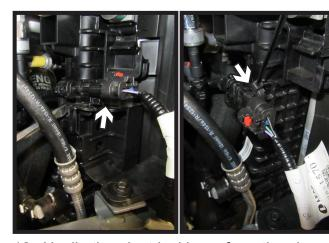
10. Unclip the electrical loom from the shroud on the passenger side of the vehicle (left). Then using a provided zip tie, connect the loom to the plastic behind the shroud as shown (right) so that it out of the way when removing the shroud piece.
