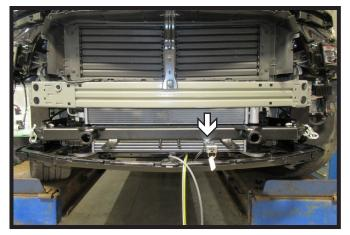
24. **Optional**: Mount the breakaway switch to the breakaway bracket with the provided 1/4" bolt and nut before reinstalling the fascia.
