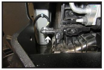
Unplug the electrical connection on the passenger side of the vehicle to allow for support plate installation. It will be reconnected later.
