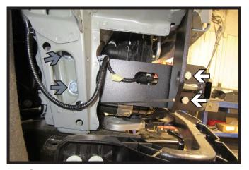
19. Slide support plate onto the vehicle toward the inside of the frame and baseplate. Start two (2) 3/8" bolts (white) with nylon lock nuts into front holes. Then start two (2) 1/2" bolts (gray) with lock washers, flat washers, and wire nuts in back holes. Tighten back 1/2" bolts then front 3/8" bolts. Do this on both sides of the vehicle.
