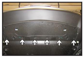
Using a 7MM socket, remove the six (6) bolts from the underside of the fascia.
