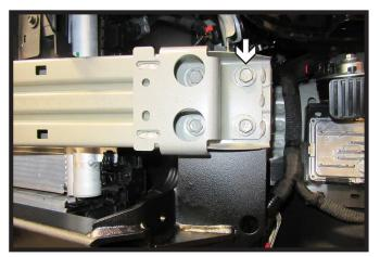
13. Slide the baseplate onto the vehicle between the frame and the bumper. Start one (1) existing 10MM bolt in the top outer hole. Do this on both sides of the vehicle. Ensure the holes on the bumper line up with the baseplate.
