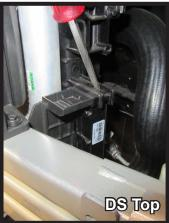
11. Using a flat screwdriver, release the four (4) clips attaching the shroud piece to the vehicle. Remove shroud and set aside, it will not be reinstalled.
