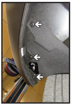
5. Using a T15 Torx, remove the three (3) bolts from the bottom of the fascia in front of the tire. Do this on both sides of the vehicle.
