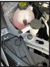
9. Using a 10MM socket, remove the two (2) nuts (white), one (1) bolt (gray), and one (1) push pin (black) from the windshield washer fluid reservoir on the passenger side of the vehicle. Disconnect and plug all lines. Remove reservoir and set aside to be reinstalled later.
