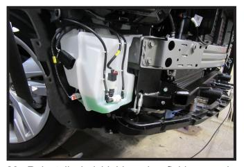
23. Reinstall windshield washer fluid reservoir, reconnecting all lines.
