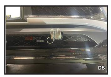
25b. **Fascia Style 2**: Hold the fascia as close to its original position and mark. Using a reciprocating saw trim each side of the fascia as shown to allow room for the baseplate and
