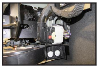
20. Reattach electrical loom to frame on the driver side of the vehicle.
