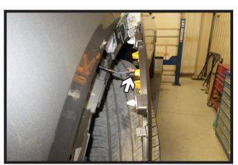
3. Pull back the wheel well trim past the fascia joint. Disconnect the one (1) electrical connection. Prop trim way from the vehicle using a soft cloth. Do this on both sides of the vehicle.
