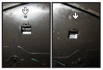
6. Using a T15 Torx, remove the two (2) bolts, one (1) on each side, from the bottom of the fascia.
