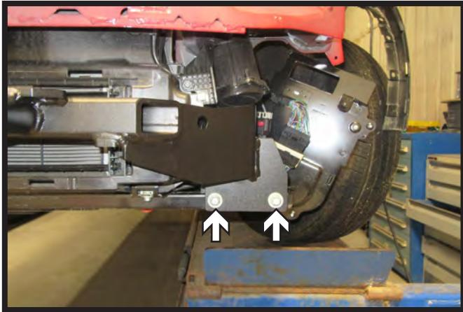
21. Slide baseplate onto vehicle. Start the two (2) existing bolts with washer into the bottom holes on the driver side of the vehicle. Leave loose.
