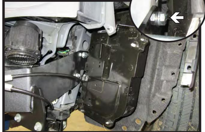
35. Reinstall the black box onto the driver side of the vehicle. Reattach the wire loom to the bottom bolt on the backside. If the box touches the baseplate bolt head, bend back plate slightly to create clearance (inset).
