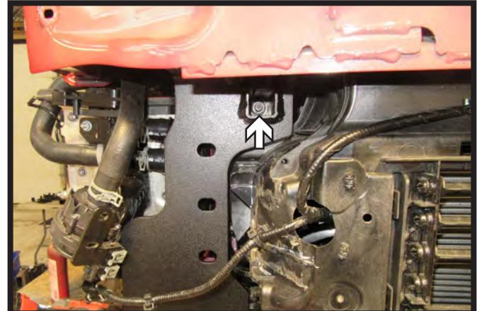
18. Reinstall the one (1) existing nut in to tube hole.
