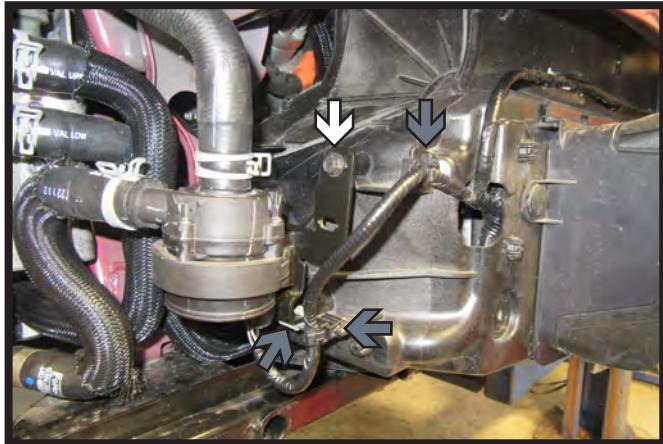
9. Using an 8MM socket, remove the one (1) bolt (white) from the bracket on the passenger side of the vehicle. Using a flat head screw driver unclip the bottom of the bracket and wire loom (gray). Let bracket hang to be reinstalled later.
