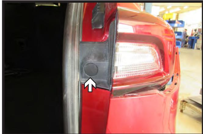
1. Remove the bolt cover from the tail light housing. Do this on both sides of the vehicle.
