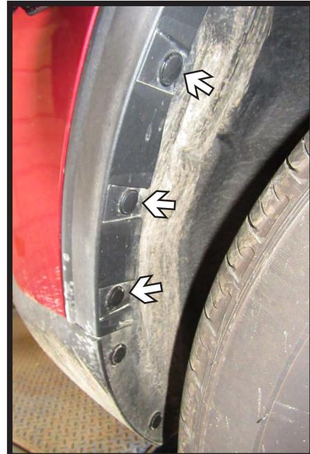
2. Remove the three (3) push pins from along the edge of the rear wheel well. Do this on both sides of the vehicle.
