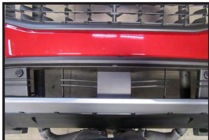
36. Remove the two (2) horizontal slats as shown to allow room for the removable tabs and convenience links.
