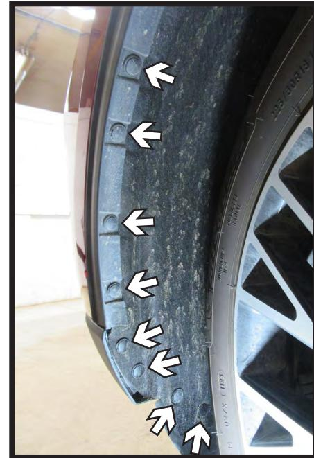
2. Remove the eight (8) push pins from along the edge of the wheel well. Do this on both sides of the vehicle.
