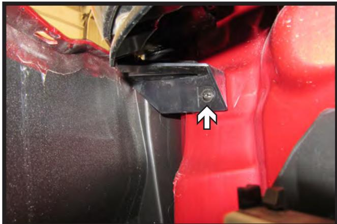
5. Using a T25 Torx, remove the two (2) bolts from the tail light housing. Remove housing and install tail light wiring kit per manufacturer's instructions. Reinstall tail light housing, rear panel and push pins. Do this on both sides of the vehicle.
