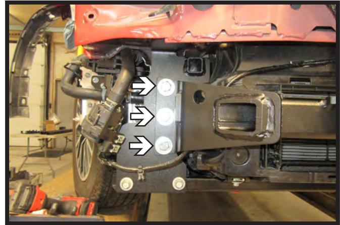
22. On the passenger side of the vehicle, start the three (3) 1 1/2" x 1-1/2" bolts with washers and nylon lock nuts. Leave loose.
