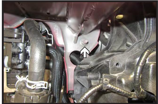
10. Using a 15MM socket with extension, remove the one (1) nut on the passenger side of the vehicle.
