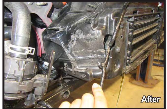
15. Using a reciprocating saw, shave the ribs on the passenger side of the vehicle as shown so they are flush with the shutter housing to allow clearance for the baseplate.
