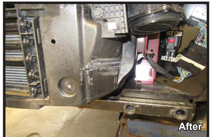
16. Using a reciprocating saw, shave the rib on the driver side of the vehicles as shown so it is flush with the shutter housing to allow clearance for the baseplate.
