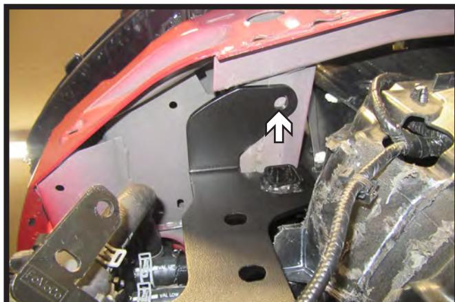
19. Using a 1/2" drill bit, drill hole in frame using the baseplate as a template.
