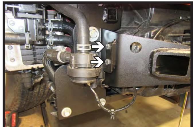
24. Using two (2) 1 1/4" x 1-1/4" bolts with nuts to attach bracket to the baseplate on the passenger side of the baseplate.
