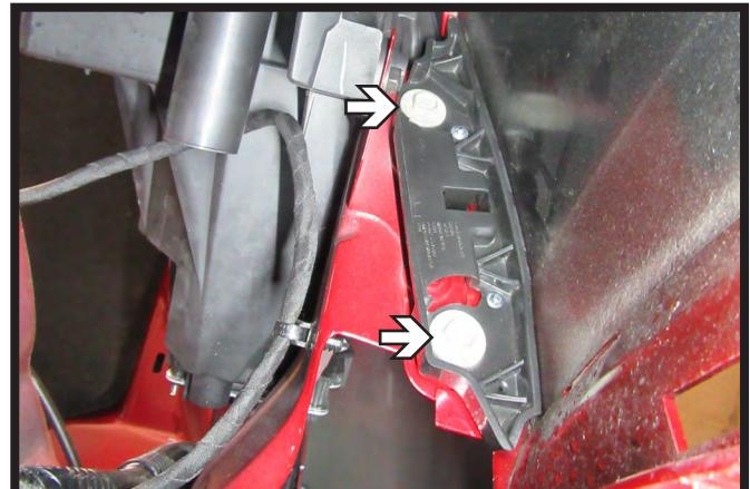
4. Pull back the wheel well liner. Using a 10MM socket, remove the two (2) bolts from the fascia joint. Do this on both sides of the vehicle.
