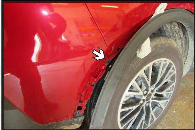
3. Pull back the wheel well trim and hold in place with a soft cloth. Remove the one (1) push pin from the rear panel joint. Do this on both sides of the vehicle.
