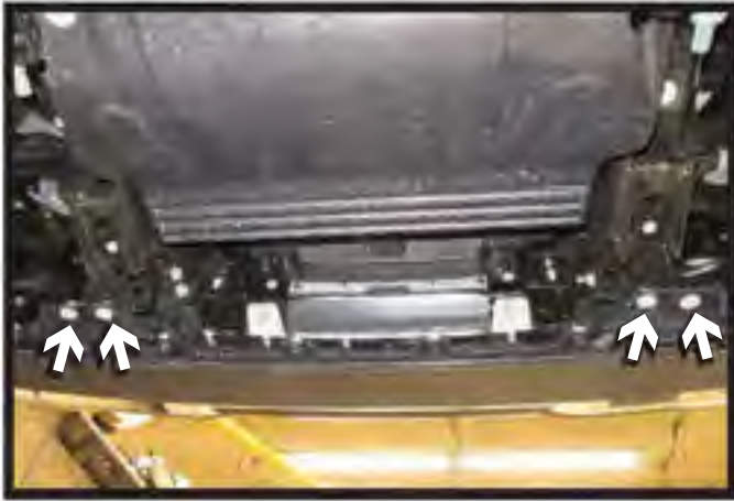
15. Using a 10MM socket, remove the four (4) bolt from the underside of the vehicle.
