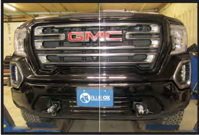
7a. Reinstall the bumper, fascia, fascia cover and reconnect all electrical.
