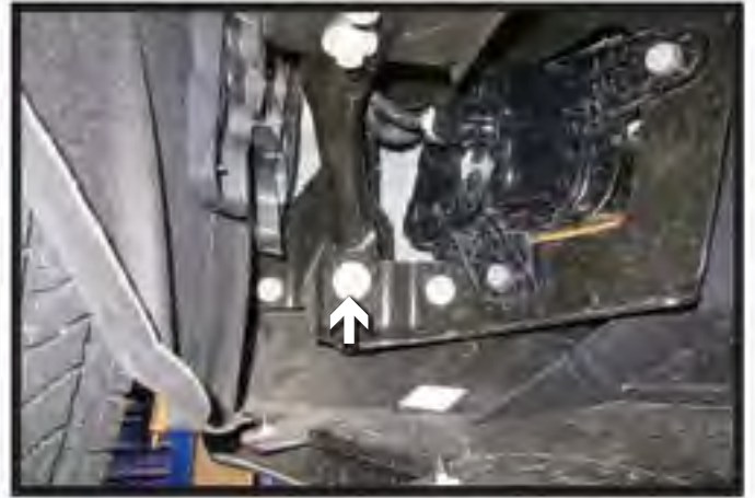
16. Using a 15MM socket, remove the one (1) bolt attaching the bracket. Do this on both sides of the vehicle.
