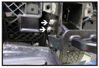
Using an 18MM socket, remove the two
