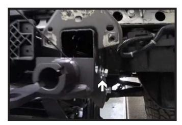
21. Rotate baseplate upward and start 1/2" bolt with hardware in the outer front hole. Do this on both sides of the vehicle.
