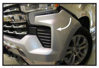
6. Starting on one side of the vehicle, lift and pull the center fascia piece way from the vehicle. Then unsnap piece across the front of the vehicle and finally lifting and pulling piece away from other side. Set center fascia piece aside to be reinstalled later.
