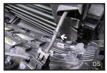
8. As the grille piece is removed, unplug the wire loom on the passenger side of the vehicle and disconnect the washer line for the camera on the driver side of the vehicle. Remove grille from the vehicle and set aside to be reinstalled later.
