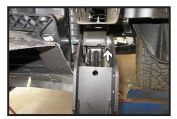
20. Slide baseplate onto tow hook housing so that the back slotted hole of the baseplate lines up with back hole on housing. Insert the one (1) 1/2" x 5" bolt with washers on the outside and three (3) spacer washers as shown. Leave loose at this time. Do this on both sides of the vehicle.
