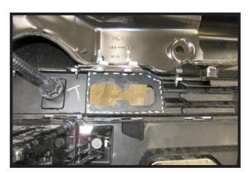
28. Using a reciprocating saw, trim the indicated area around tow hook opening on the back of the bumper to allow clearance for baseplate. Do this on both sides of the vehicle. Reinstall bumper and reconnect electrical.
