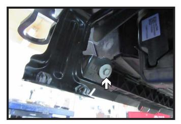
17. Using a 10MM socket, remove the one (1) bolt from the back of the lower shutters on the driver side of the vehicle.
