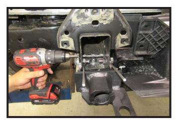
24. Using a 1/2" drill bit, drill the top rear inside hole on the passenger side of the vehicle, using the baseplate as a template. Drill straight through the tow hook housing from the rear outside hole to drill rear inside hole.
