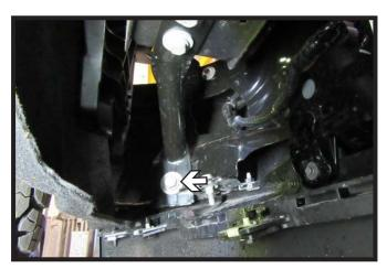
13. On the underside of the vehicle, use a 15MM socket to remove the one (1) bolt holding the bracket. Do this on both sides of the vehicle.
