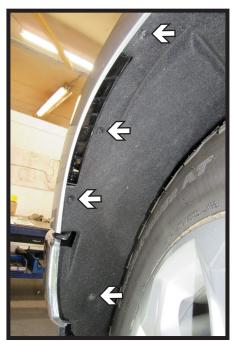
4. Using a T15 Torx, remove the four (4) bolts along the wheel well edge. Do this on both sides of the vehicle.
