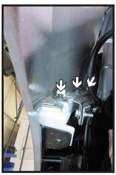
5. Pull back the wheel well liner. Using a 7MM socket, remove the three (3) bolts from the fascia joint. Do this on both sides of the vehicle.
