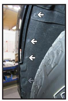
3. Using a 5.5MM socket, remove the three (3) bolts (white) and one (1) push pin (gray) from along the wheel well edge. Do this on both sides of the vehicle.
