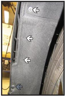
Using a 5.5MM socket remove the three
