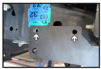
4. Using a 1/2" drill bit, drill two (2) holes in the frame using the baseplate as a template. Do this on both sides of the vehicle.
