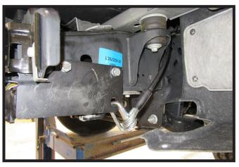
6. Attach the permanent baseplate safety cables to the provided convenience link on the baseplate. The photo above shows the recommended installation of the cables to frame of vehicle. Additional options may interfere with suggested mounting; in this case, secure the cables to a solid piece of the frame as described in the General Information sheet. Be sure the safety cables do not rub against any hoses or moving parts. Do this on **BOTH** sides of the vehicle.
