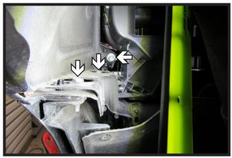
4. Pull back the wheel well liner. Using a 10MM socket, remove the three (3) bolts from the fascia joint. Do this on both sides of the vehicle
