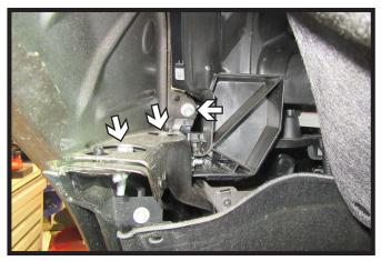
2. Pull the liner back, then using a 10MM socket remove the three (3) bolts. Do this on both sides of the vehicle.
