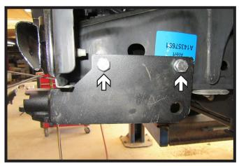
5. Install two (2) 1/2" x 1-3/4" bolts with lock washers and whiz nuts. Do this on both sides of the vehicle.
