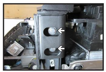
3. Hold baseplate in position and start two (2) 1/2" x 1-3/4" bolts with flat washers and lock washers on the bottom and whiz nuts on the top. Push baseplate against frame and tighten bolts. Do this on both sides of the vehicle.
