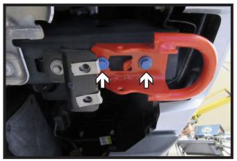
Using a 15MM socket, remove the two
