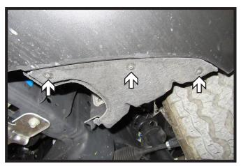
8. Using a 5.5MM socket, remove the three (3) bolts from the underside of the fascia in front of the tire. Do this on both sides of the vehicle.
