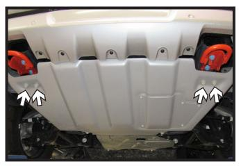
5. Using a 13MM socket, remove the four (4) bolts from the belly pan, two (2) on each side.
