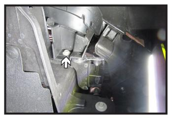
Using a 10MM socket, remove the one (1) bolt from underneath the vehicle in front of the radiator. Do this on both sides of the vehicle.
