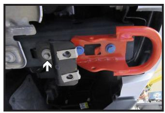
7. Using a 13MM socket, remove the one (1) bolt from the belly pan bracket. Remove bracket and set aside to be reinstalled later. Do this on both sides of the vehicle.
