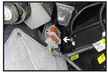
Disconnect electrical connection on the driver side of the vehicle.
