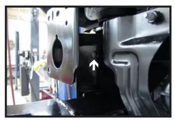
8. Using a 1/2" drill bit, drill the front inside hole using the baseplate as a guide. Install one (1) 1/2" bolt with lock washer and whiz nut. Do this on both sides of the vehicle.
