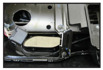
Using a reciprocating saw, remove the indicated area on the back side of the fascia to allow room for the baseplate. Do this on both sides of the fascia.
