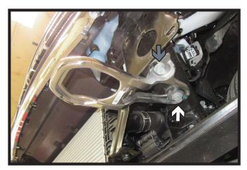
4. **Trucks with Tow Hooks:** Using an 18MM socket remove the front bolt (gray), and then using a 21MM socket remove the back bolt (white) attaching the tow hook to the frame. Do this on both sides of the vehicle. The tow hooks will not be reinstalled.
