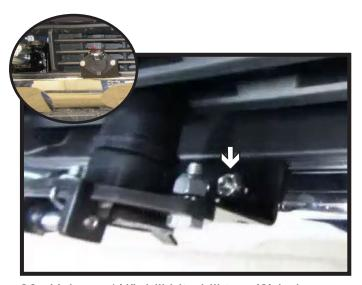
20. Using a 1/4" drill bit, drill two (2) holes on the passenger side of the vehicle using the electrical bracket as a guide. Insert two (2) 1/4" bolts with hardware.
