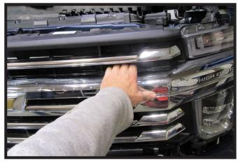
8. Grab the grille near the top and pull firmly away from the vehicle. Unsnap remaining clip near the bottom center of the grille. Remove grille and set aside to be reinstalled later.
