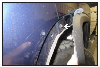
5. Unclip the front half of the wheel well trim. Prop trim away from vehicle using a rag or soft material to prevent scratching. Using a 7MM socket, remove the one (1) bolt from the fascia joint. Do this on both sides of the vehicle.
