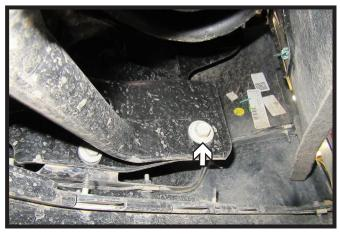
Using a 15MM socket, remove the one
