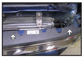
3. Using a 10MM socket, remove the two (2) bolts from the top of the fascia. Do this on both sides of the vehicle.
