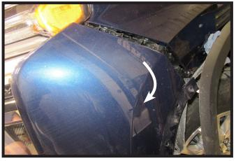
Grab fascia in the wheel well and pull outward firmly to remove corner of center fascia piece. Do this on both sides of the vehicle. Remove center fascia piece and set aside to be reinstalled later.
