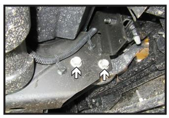
Using an 18MM socket, remove the two (2) bolts from the tow hook. Do this on both sides of the vehicle. Remove tow hooks, they will not be reinstalled.
