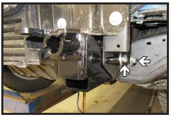
14. Slide the baseplate into the frame. Insert two (2) 1/2" bolts with lock washers, flat washers, and spacers. Do this on both sides of the vehicle.
