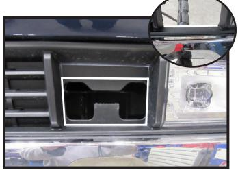
18. Trim the tow hook opening as indicated to allow room for the baseplate. Then trim the bottom inner side at an angle as needed (inset).
